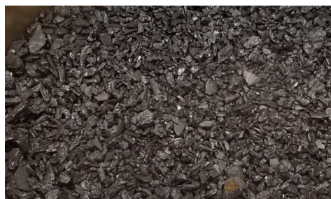
Fig. 2. Cerium metal after hydrogenating step.
