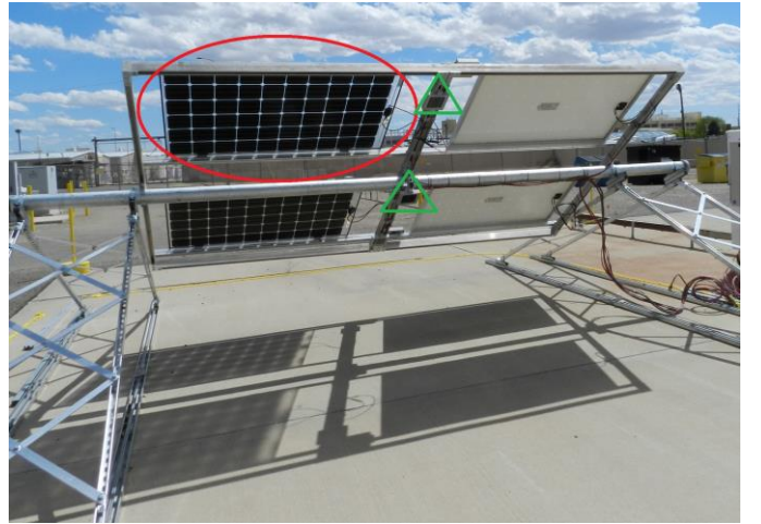
Fig. 10. Bifacial PV module under test circled in red. Rear irradiance reference cells shown with green triangles
