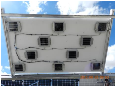
Fig. 2. Sandia's high spatial resolution rear irradiance module. A sensor with PV module form factor and ten reference cells measuring rear irradiance
