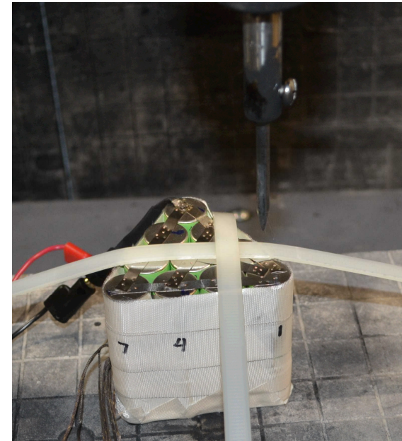
1S10P Battery: Failure point on edge cell
