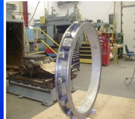
Electron Beam Freeform Fabrication (Accleron Inc.)
