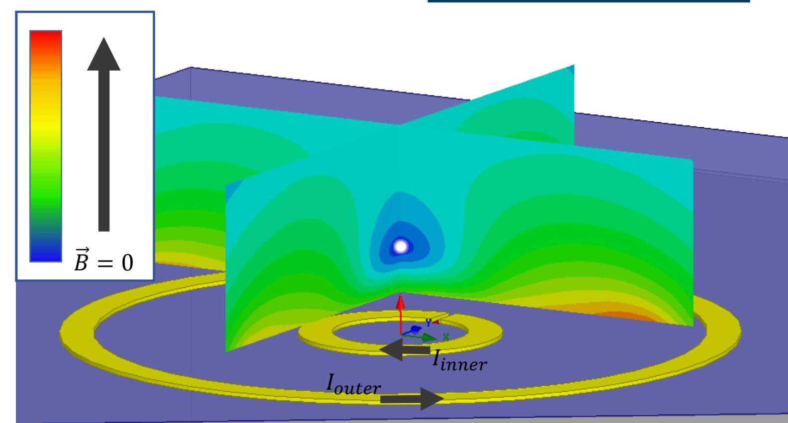
Create a strong magnetic field gradient to couple the ion qubit and motion
