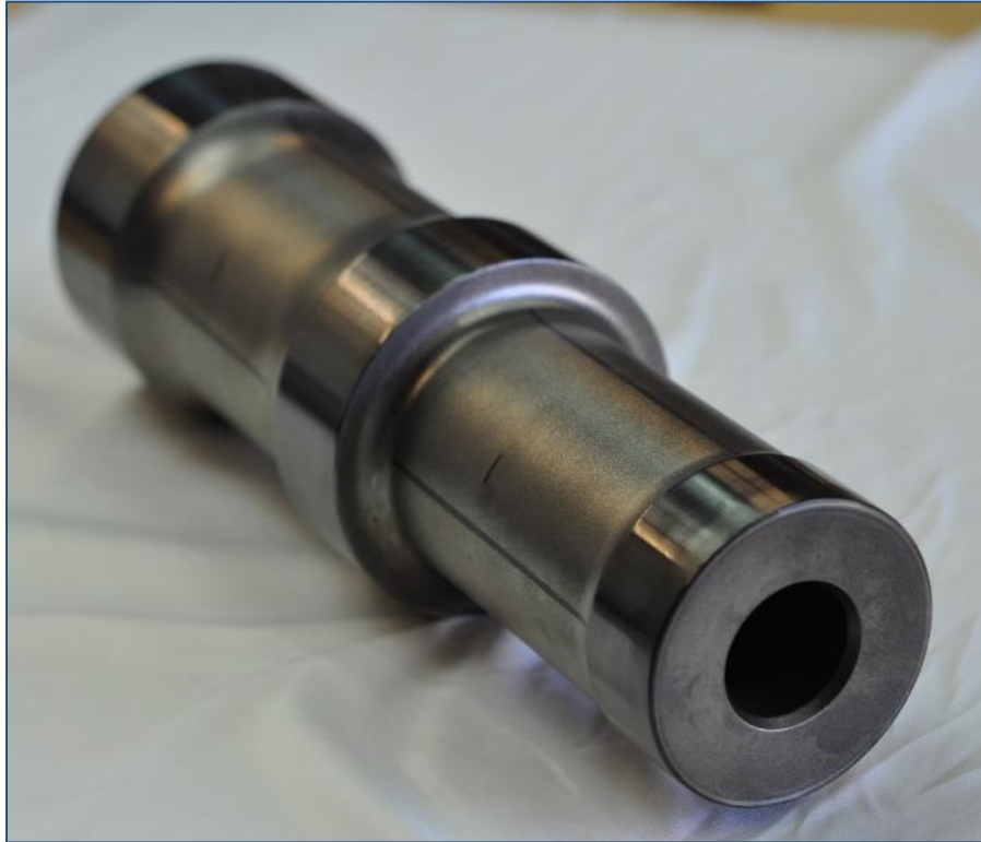
Figure 26. LT piston with DLC coating applied
