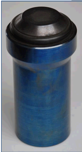
Figure 32. Check valve tempering temperature color change
