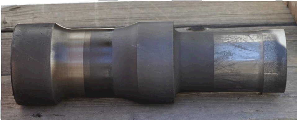
Figure 24. Piston with no lubrication at 400°F
