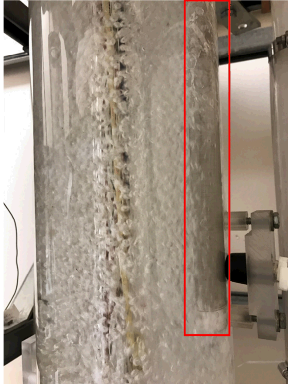
Figure 11: Photo of the tool in two-phase flow
