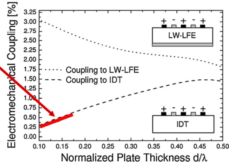
Two fundamental subsets of Lamb-wave Contour mode resonators (CMR) – 1) top electrode interdigitated transducer (IDT) and 2) IDT top electrode with floating lower electrode.
