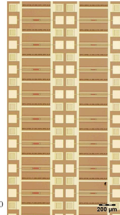
With CMR, a wide range of resonances can be achieved on the same wafer, and on the same die. Above is a die of resonators created in 750 nm thick AlN.
