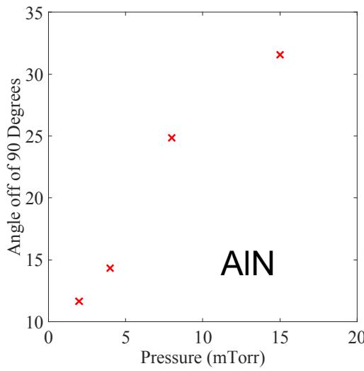
Control over the sidewall angle is controlled by the chamber pressure.
