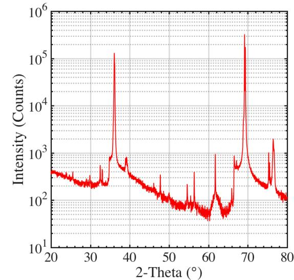
XRD scans of AlN film with a (002) peak located at  $36.082^{\circ}$  and a rocking curve FWHM of  $2.248^{\circ}$ .
