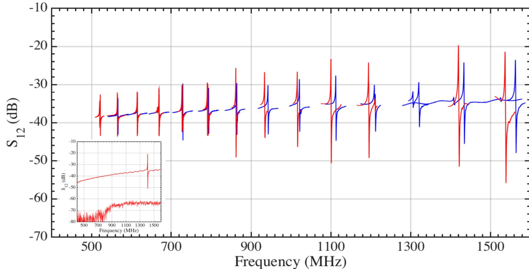
Red is the ScAlN resonators and blue is AlN. A clear improvement in resonator Q and  $k^2_{\text{eff}}$  is visible.
