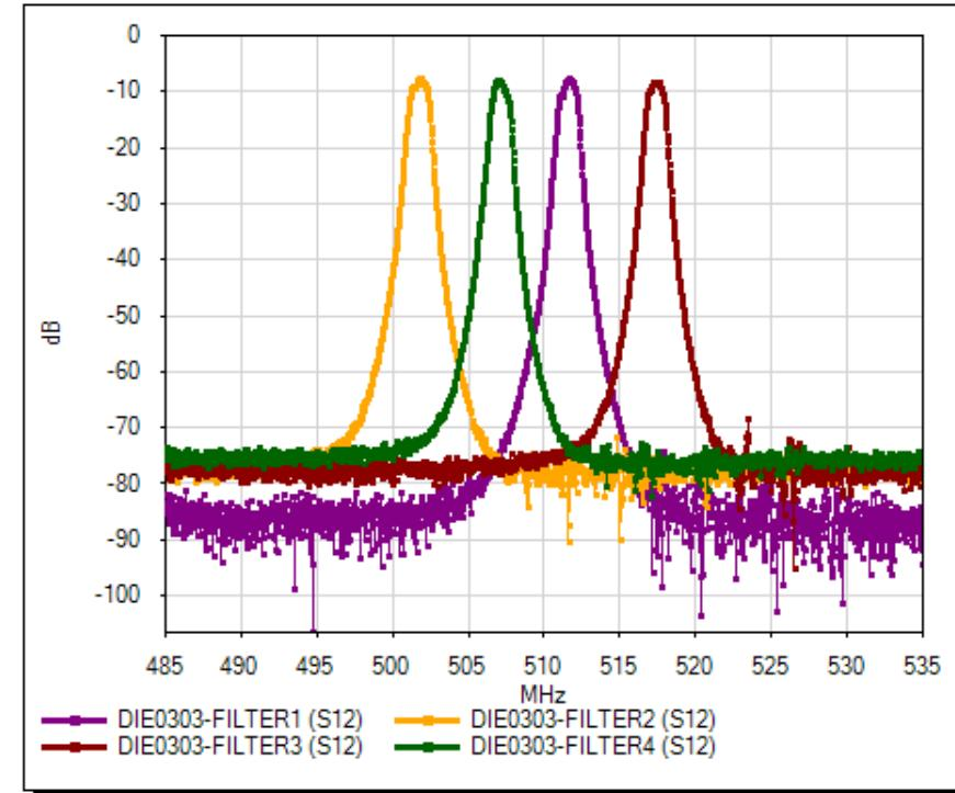
Small changes in the lithographic layout of the CMRs, can control the bandpass frequency. Other piezoelectric device designs require changes to the film thickness; this is less optimal.
