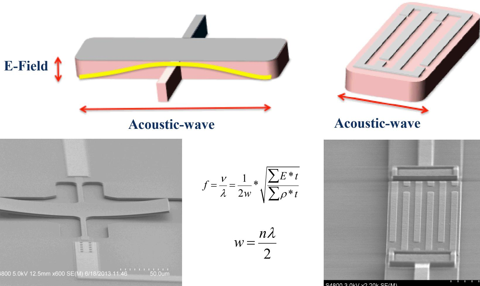
Contour mode resonators take an electric field (z axis) and create an acoustic wave (x axis) using the piezoelectric properties of a film (AlN).
