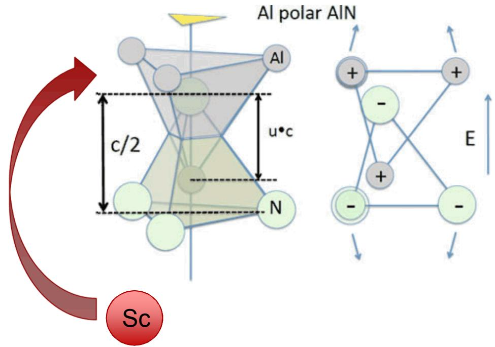
Substitutional replacement of Al with Sc, is expected to increase the ionic displacements in electric fields.
