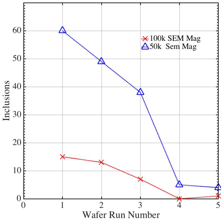
For a cassette load of wafers, running 4 to 5 dummies ahead of the device wafers drives the inclusion count to acceptable levels. This suggests conditioning of the target or residual gas (maybe loadlock) is needed to eliminate species.
