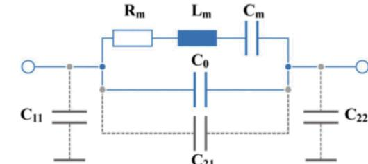
$$Z_{resonator} = \frac{1 + SR_m C_m + S^2 L_m C_m}{1 + SR_m (C_m || C_0) + S^2 L_x (C_m || C_0)} * \frac{1}{S(C_m + C_0)}$$
