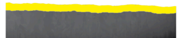
Gold plating fills in surface roughness
