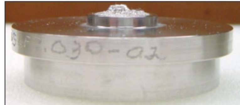
Fig. 6 — Bore and radial repaired scratches on the surface of the weld bases.
