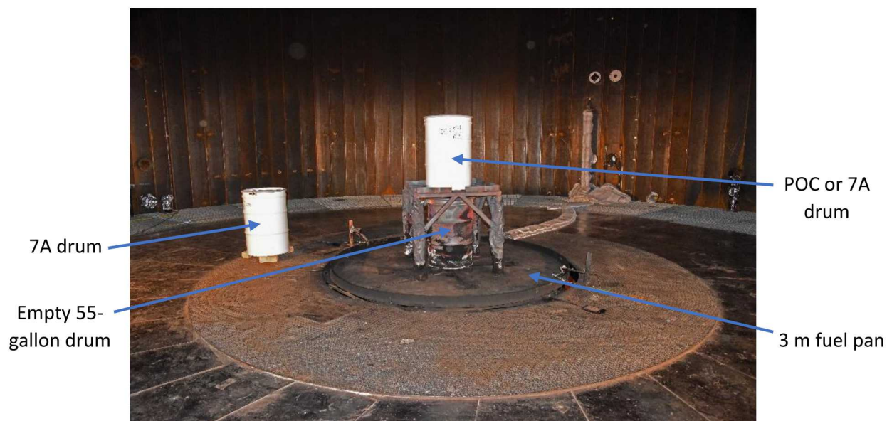
Figure 4. Typical fuel-pool/drum layout for Test #2 and Test #4 inside of FLAME.
