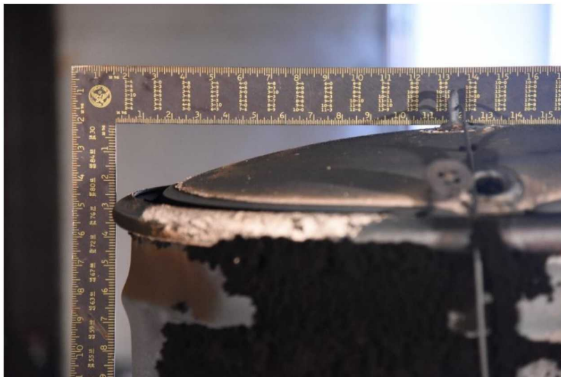
Figure 21. Bulging of POC drum in Test #1.
