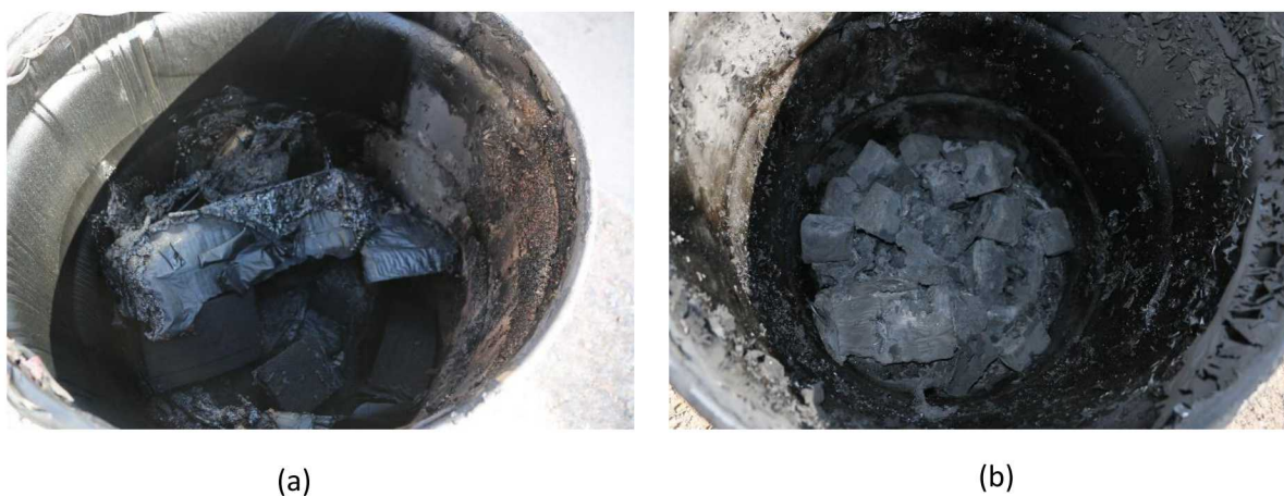
Figure 28. Remains of 7A drums for Test #4. (a) drum placed at the 35 \text{ kW/m}^2 distance, and (b) drum placed in center of pool fire.
