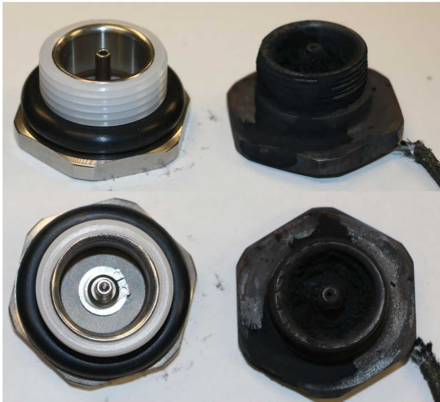
Figure 22. Comparison of new filter vs tested filter from Test #1.
