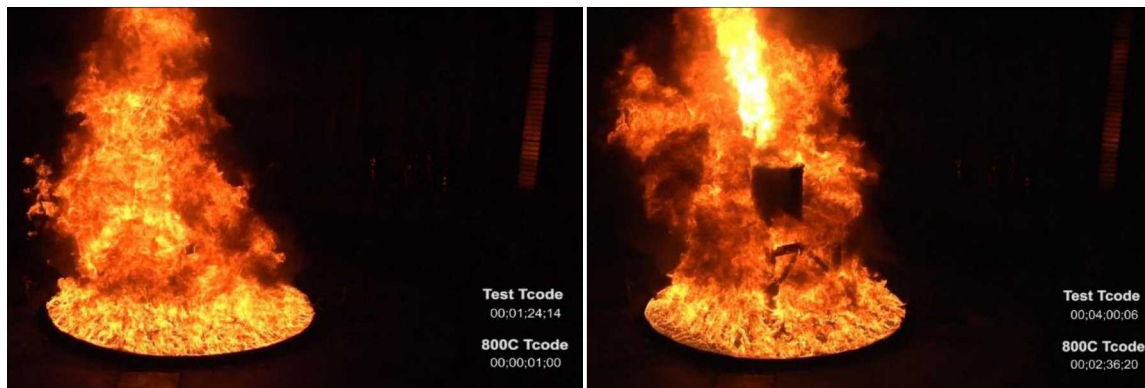
Figure 18. POC under fully engulfed fire conditions: (a) Before filter ejection and (b) after filter ejection.
