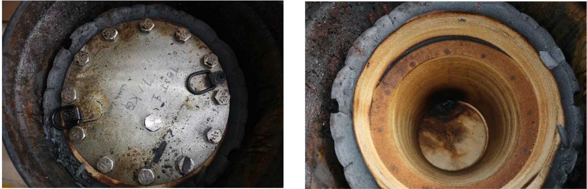
Figure 23. Internal conditions of POC from Test #1 after test completion when Celotex® top is removed.
