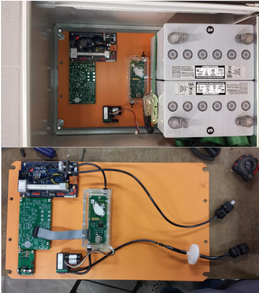
Figure 2.16: (TOP) The layout of components within the large communication nodes. The batteries take up most of the space inside the enclosure, so components were arranged to be bolted to the top of the back plate. (BOTTOM) Behind the batteries, tubing to direct the air for the active sampling is laid.
