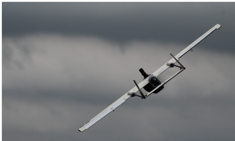
Figure 3.35: Aircraft with improved sensor mast.
