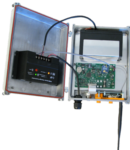
Figure 2.15: A photo depicted the internal arrangement of boards and wiring within a completed sensor node.
