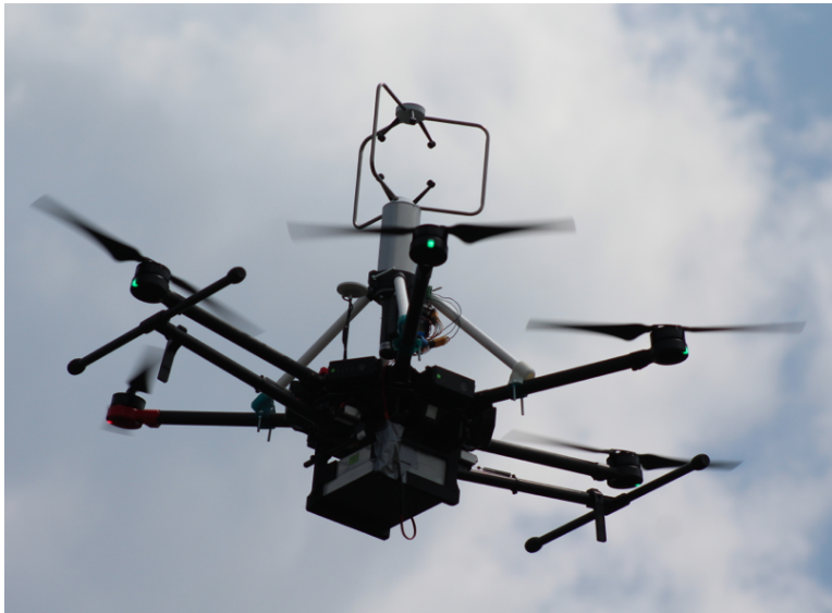
Figure 3.41: Prototype mobile eddy covariance “tower” with integrated ultrasonic sensor with \text{CO}_2 detection.
