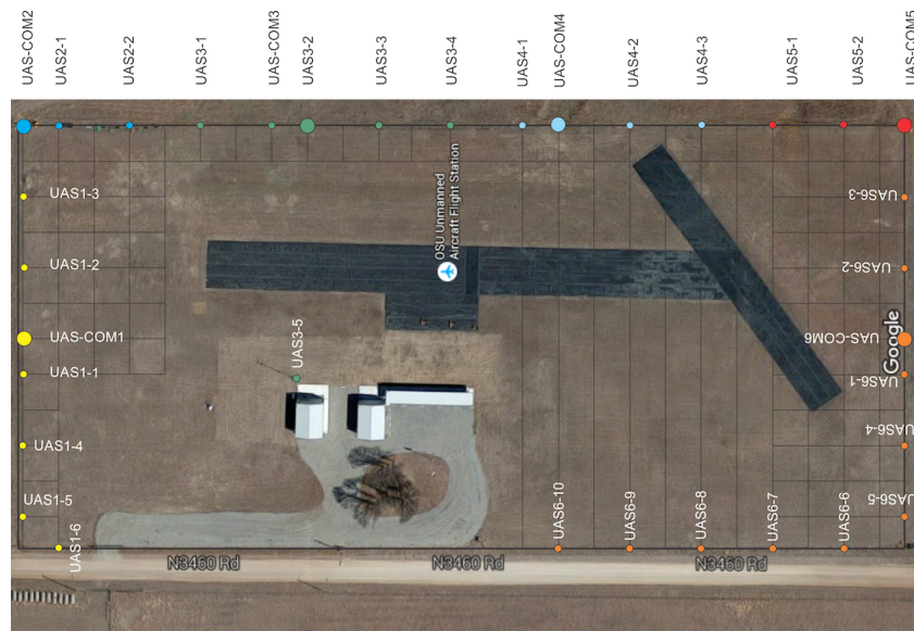
Figure 2.22: Configuration of the sensor the unmanned airport flight station. The larger circles represent communication nodes and the smaller circles are the sensor nodes.
