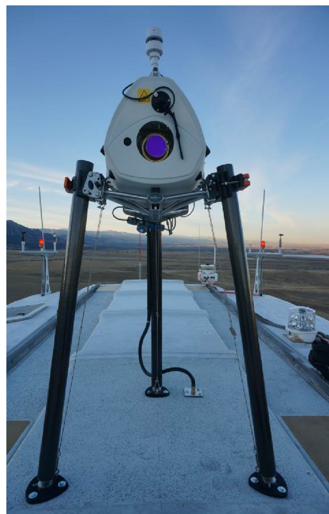
LIDAR installed on ECO110
