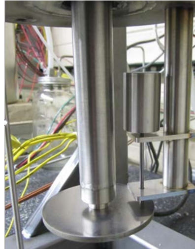
Figure 4: Pin and Weight Loaded on Disc
