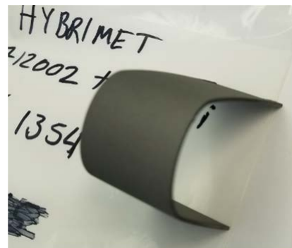
Fig 6. 0.015 HVOF HybriMet 360° bend without any spallation or cracking.
