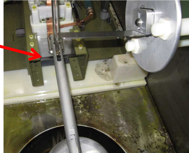
Photograph of the output swingarm on an MTG. The air-driven solenoid takes ~1 sec to actuate.
