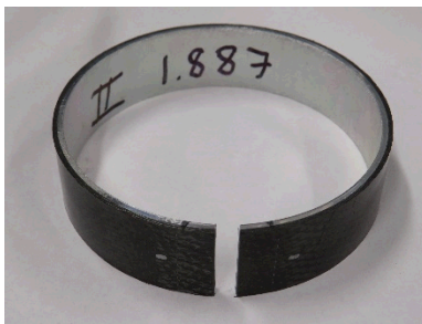
Figure 3. Bi-material cylinders at room temperature: carbon fiber composite – no skew (left), carbon fiber composite – 45^\circ skew (center), and glass fiber composite – no skew (right).
