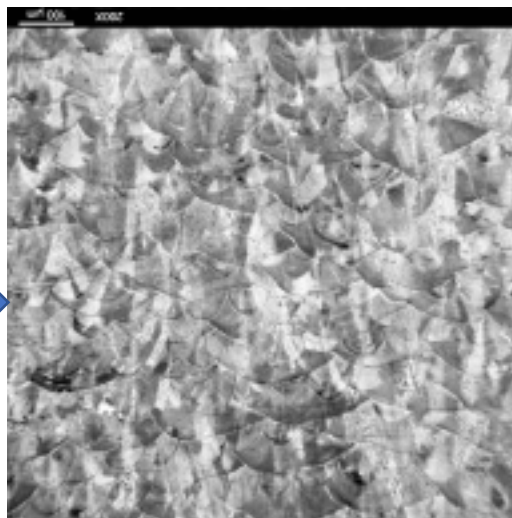
Nitric acid etched PBF hexagon
