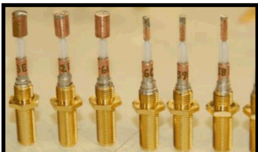
4.75mm electrode (left) 2.03mm electrode (right)
