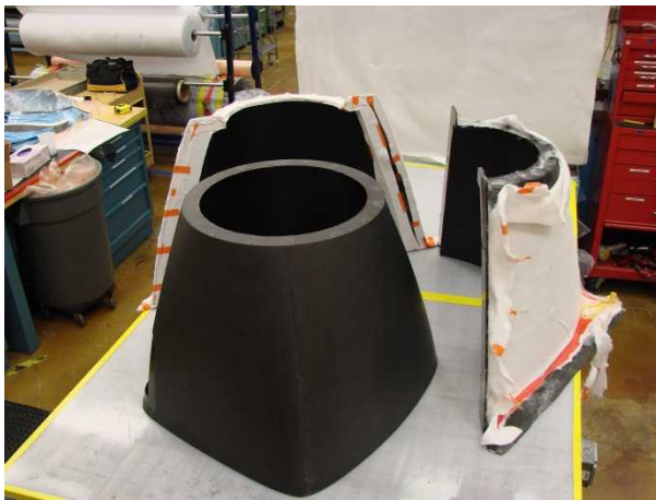
Aft Cowl Demolded and Removed from Female Tool
