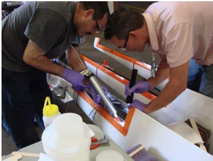
Bonding Spar and Riblet in Place
