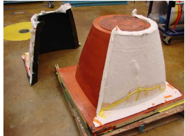
Aft Cowl Master and Female Production Tool
