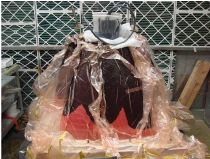
VARTM Shot - Resin Impregnating Laminate Buildup
