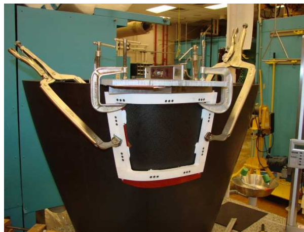
Custom Fixtures used to add Final Holes
