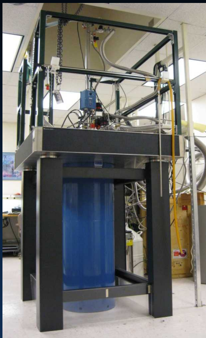
Dilution refrigerator: 10 mK
