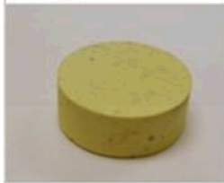
50 wt% AgI/50 wt% Glass, 500°C for 3 hr
