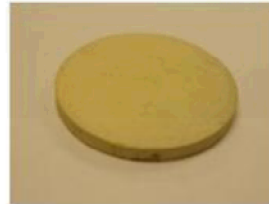
50 wt% AgI/50 wt% Glass, 500°C for 3 hr
