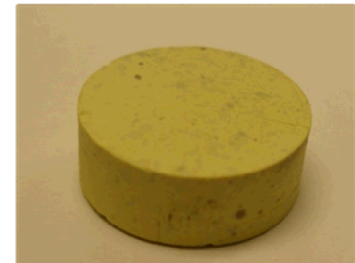
Glass/AgI-MOR pellet sintered to high density at 550°C.
