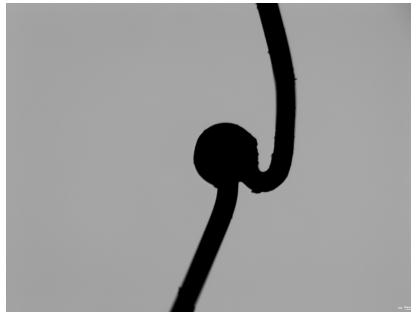
Figure 1. Backlit photograph of a commercially produced type-R thermocouple with a wire diameter of 51 \mu\text{m} , as observed under a microscope.
