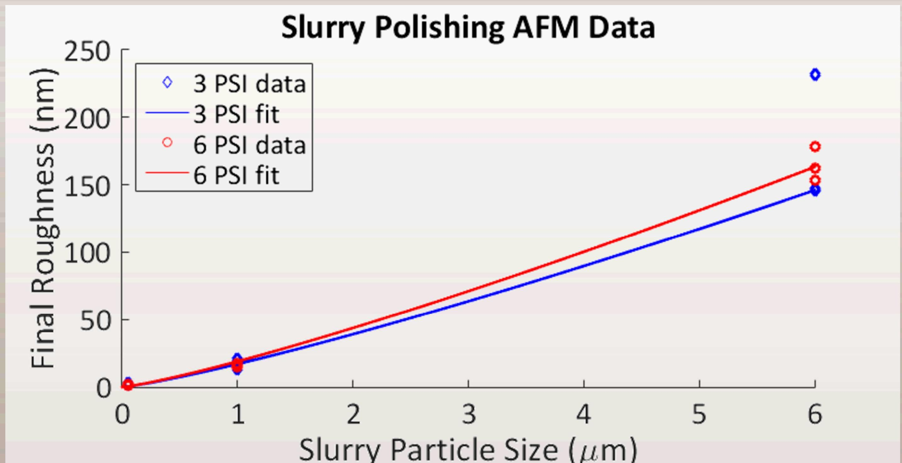
Tilt SEM of Si surface after 6PSI grind with various films (top) and surface roughness data after polish with several slurry sizes (bottom)
