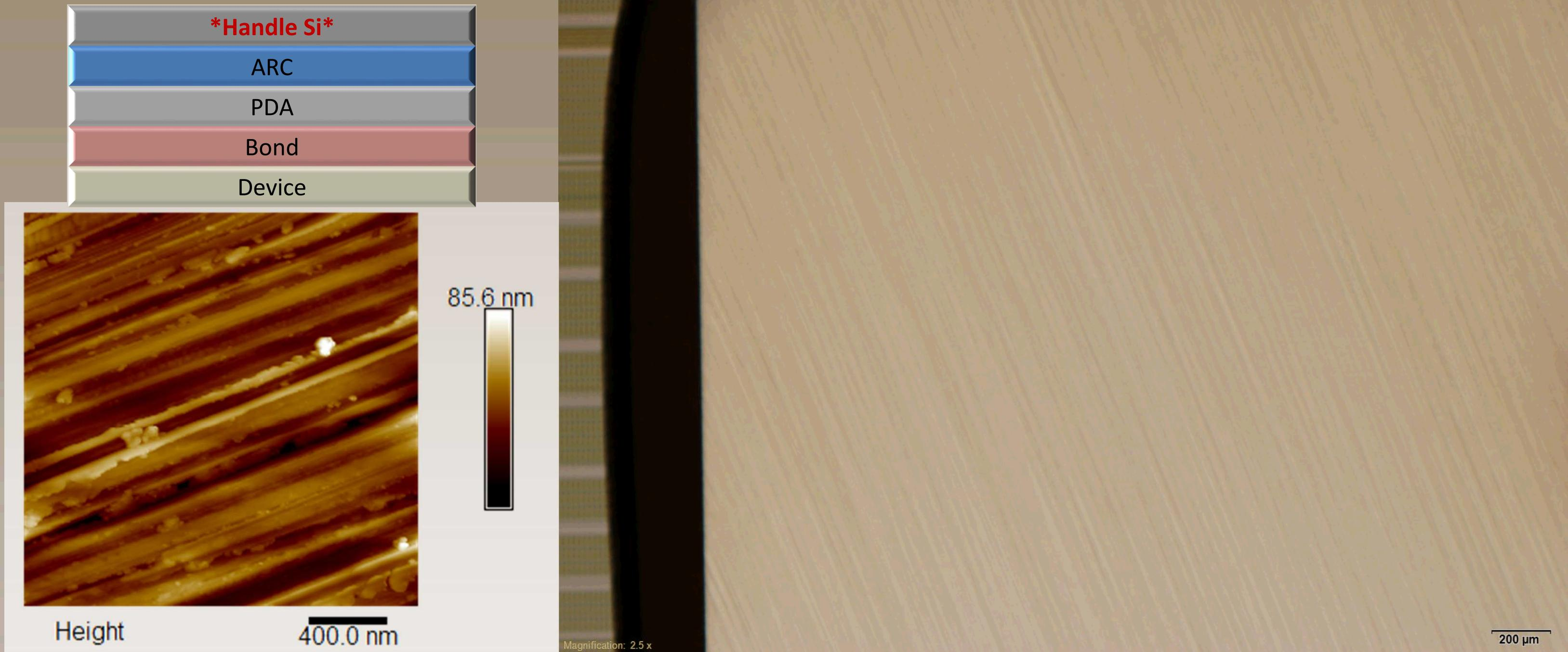
Surface roughness data (left) and optical image (right) of a part polished with initial process. Large white particles are embedded diamond.
