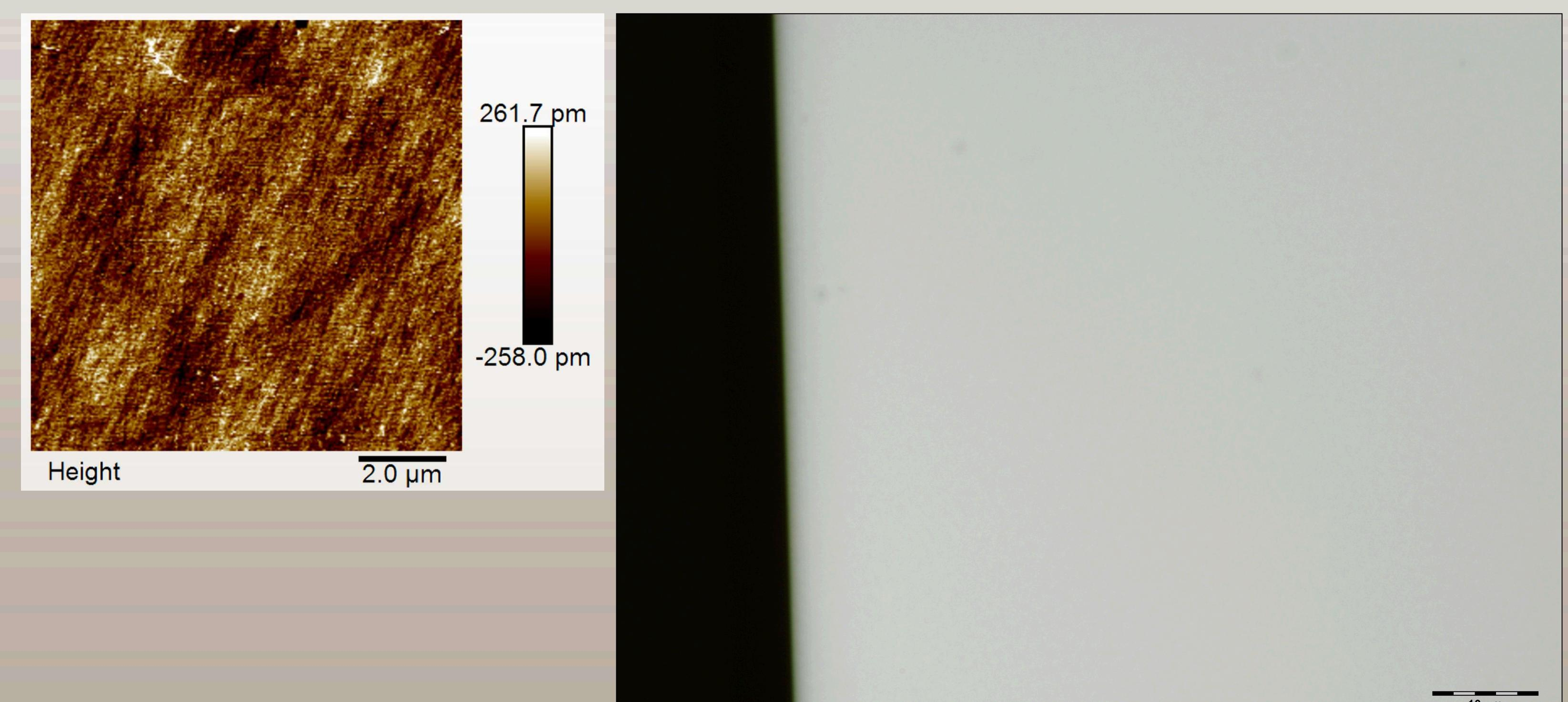
Surface roughness data (AFM) of a part polished with developed BKM (left) and an optical image of the polished surface (right)
