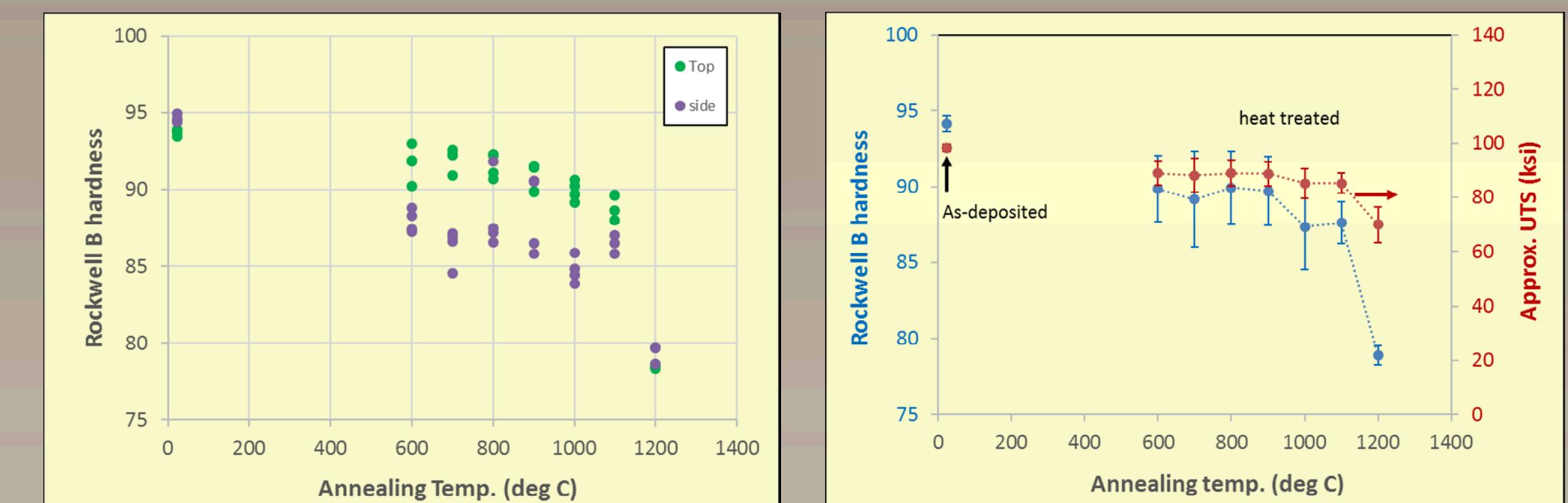
Hardness in the top-down direction was slightly, but consistently, higher than hardness measured on the side of the build. This was true for the (anisotropic) columnar grain structures produced at intermediate anneal temperatures. The as-deposited material and the 1200°C annealed samples were isotropic in both microstructure and hardness.
