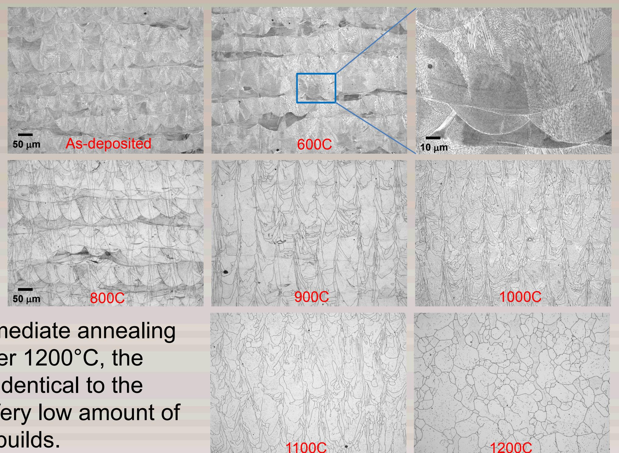
Layers of overlapping laser welds are visible. Fine-scale cellular structure is annealed out between 700 and 800°C. A roughly columnar grain structure develops at intermediate annealing temperatures. After 1200°C, the microstructure is identical to the top-down view. Very low amount of porosity in these builds.
