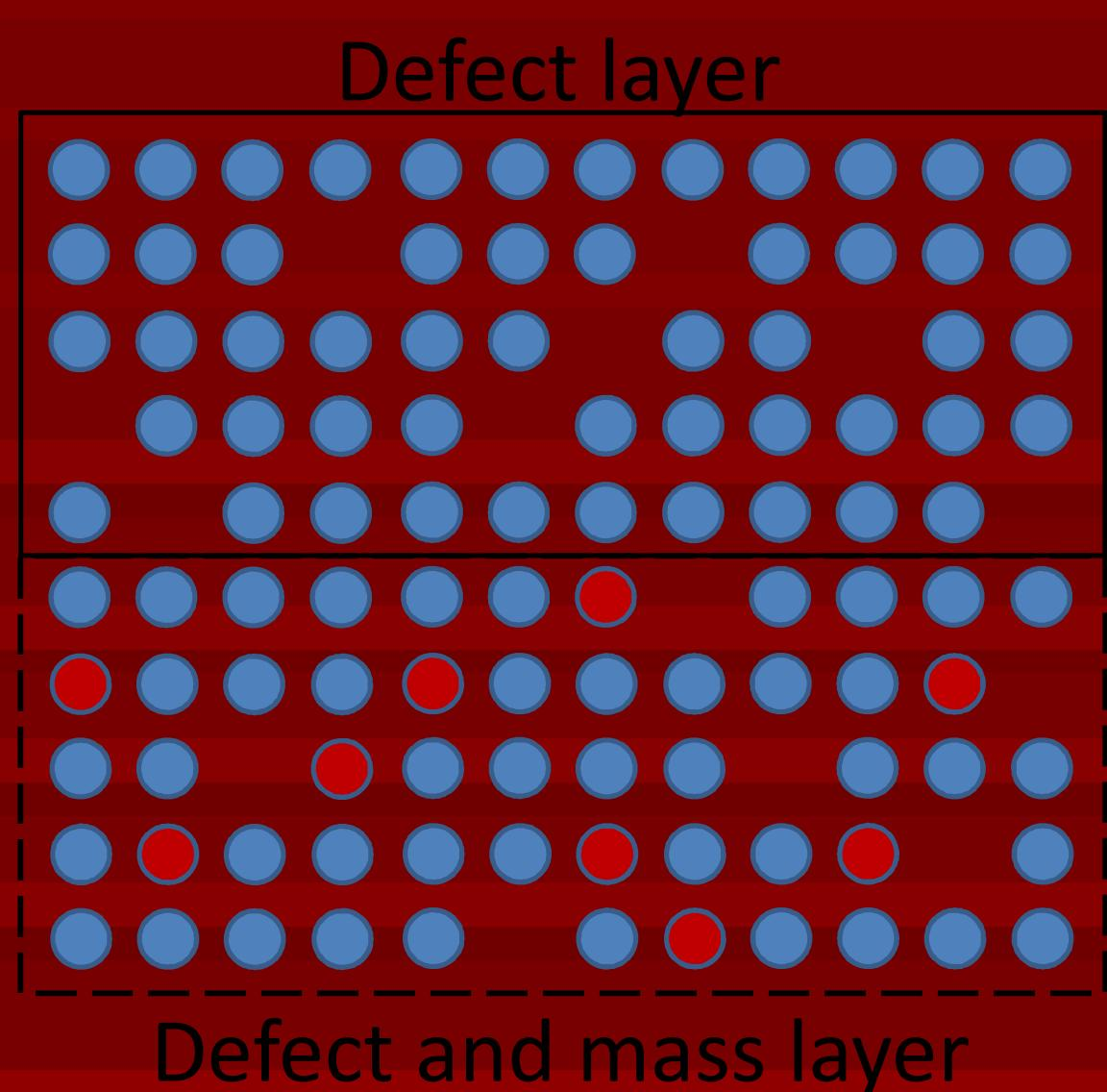
**Takeaway:** Irradiation causes defect and impurity scattering.
