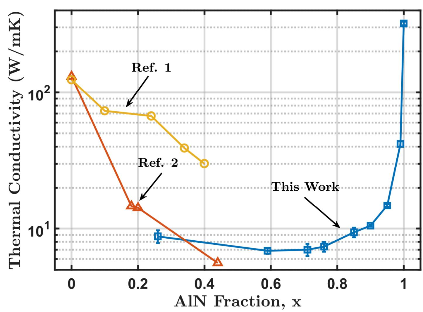
**Takeaway:** Alloying produces typical bathtub shape with disordered alloy-like magnitudes.
