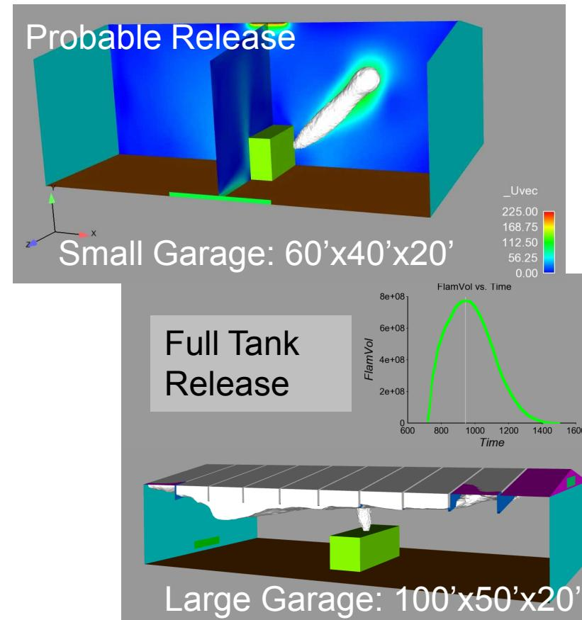
Results indicate that flammable concentrations can occur in regions not protected by NFPA 30A (lower than 18" from the ceiling). Results can be used to assess sensor placement.
