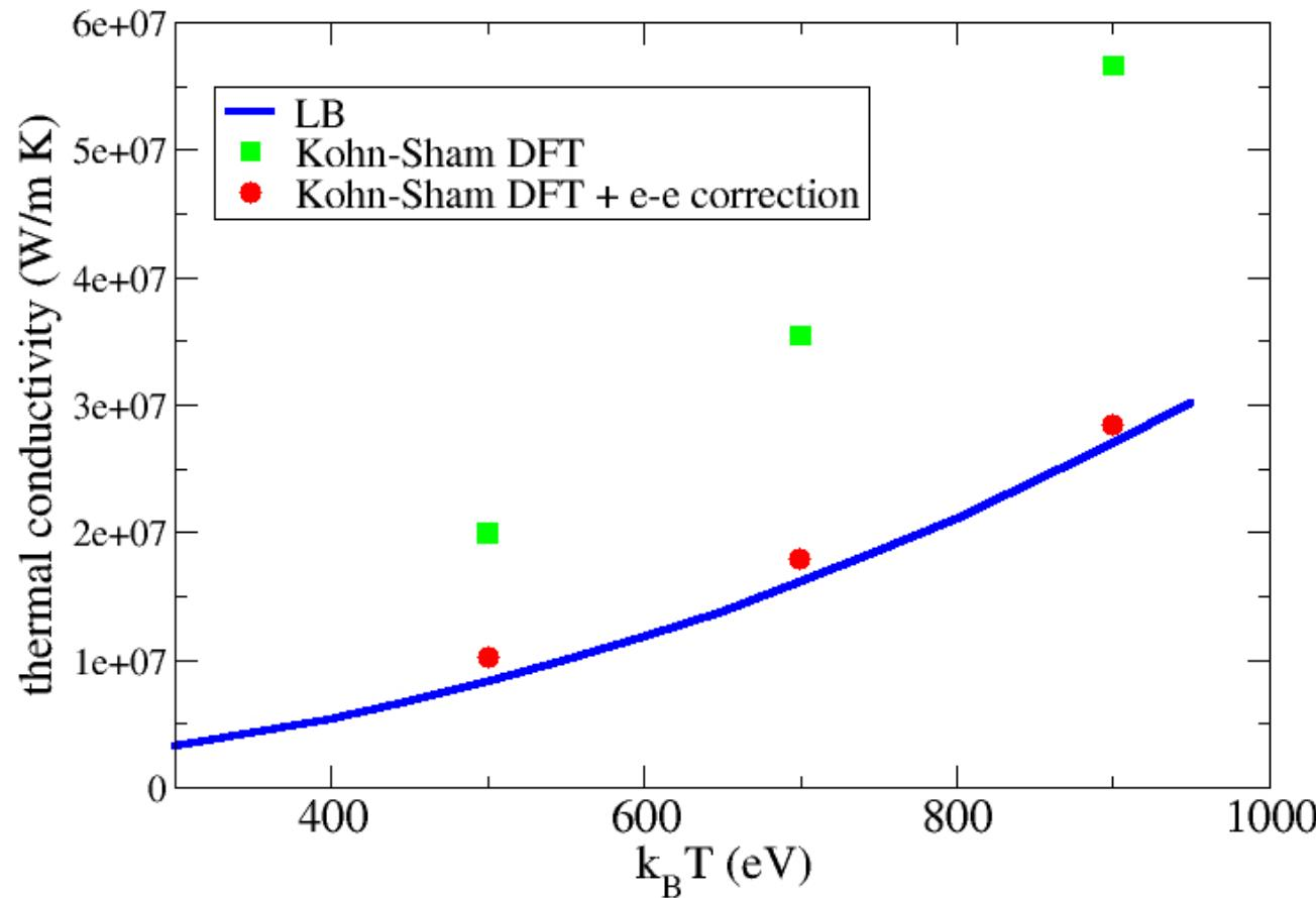
The red points show the agreement when an explicit e-e scattering correction, calculated in the Zubarev formalism (T-matrix, Boltzmann collision operator) is added to the thermal.
