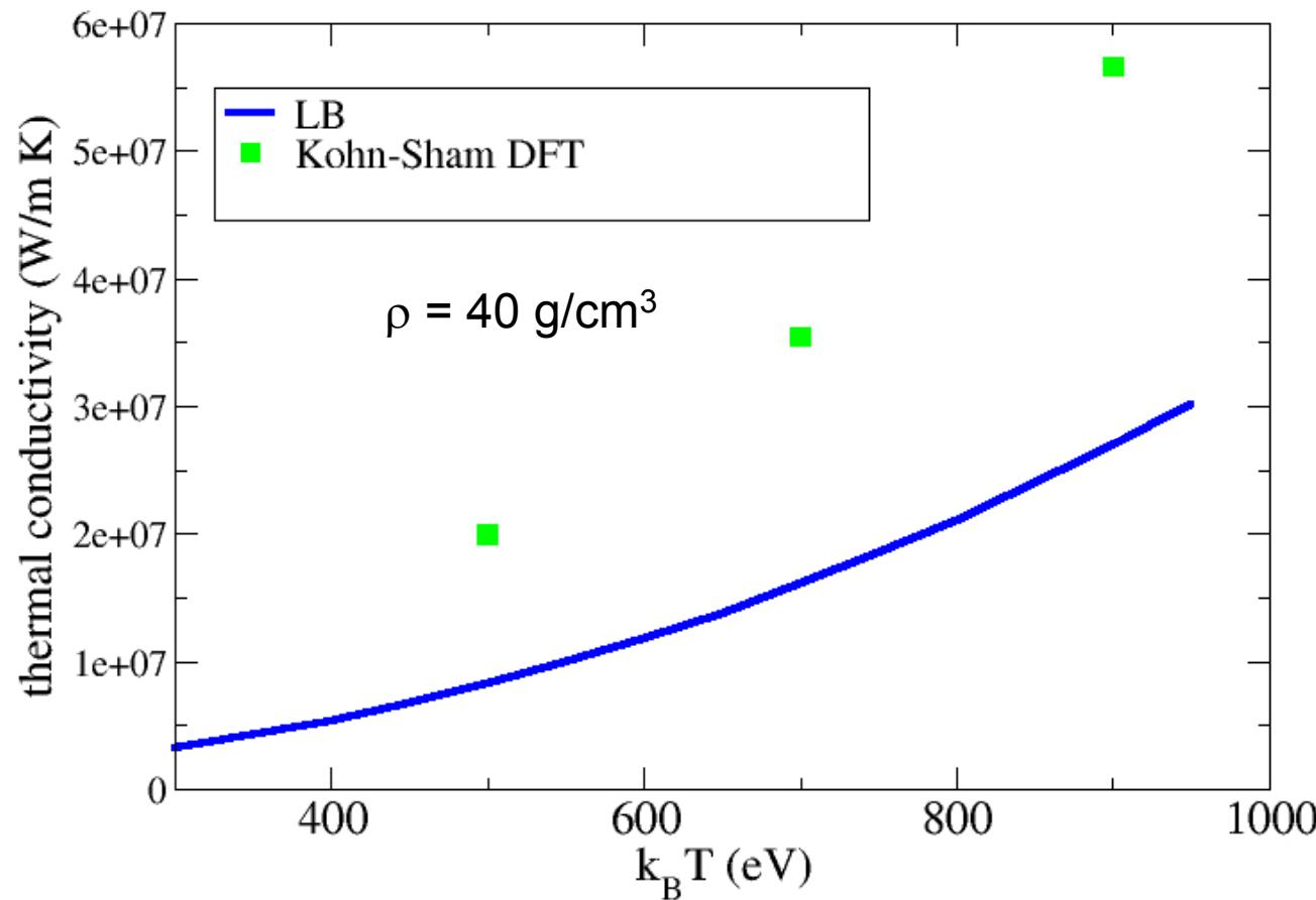
Density functional theory provides an accurate description of the electrical conductivity in the non-degenerate limit, but only partially captures the thermal transport
