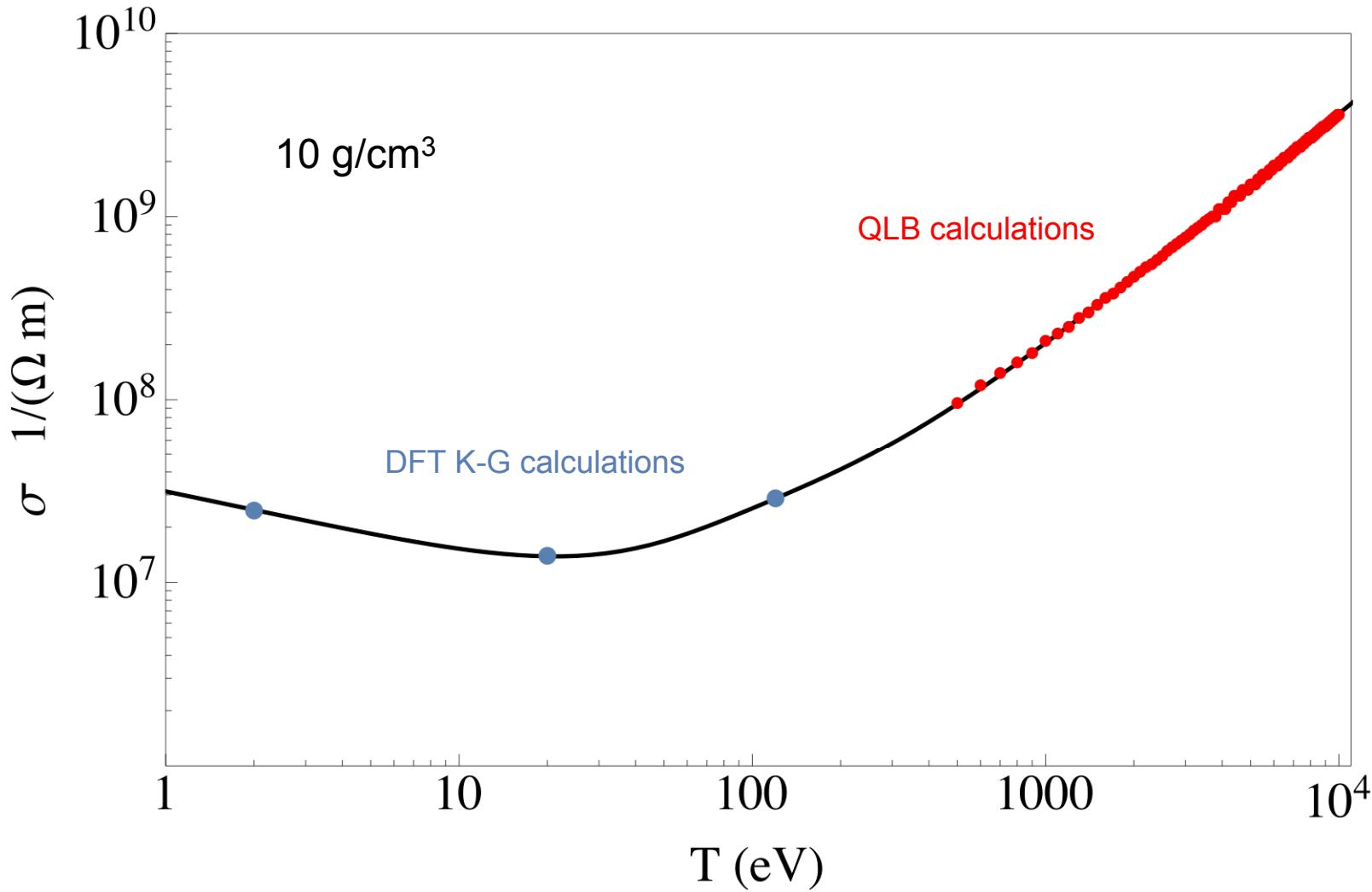
The model is tuned to our DFT Kubo-Greenwood thermal conductivity calculations in the degenerate limit
