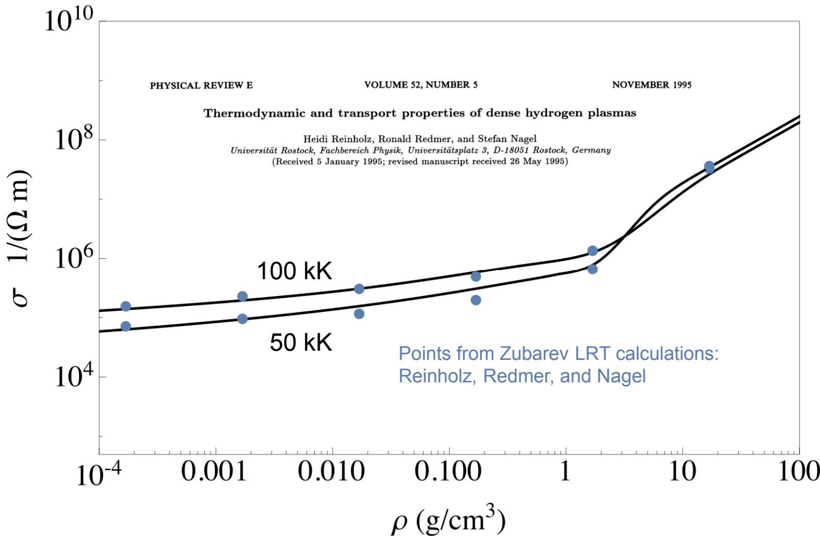
The wide-range model is in good agreement with Zubarev thermal conductivity calculations for hot expanded plasmas
