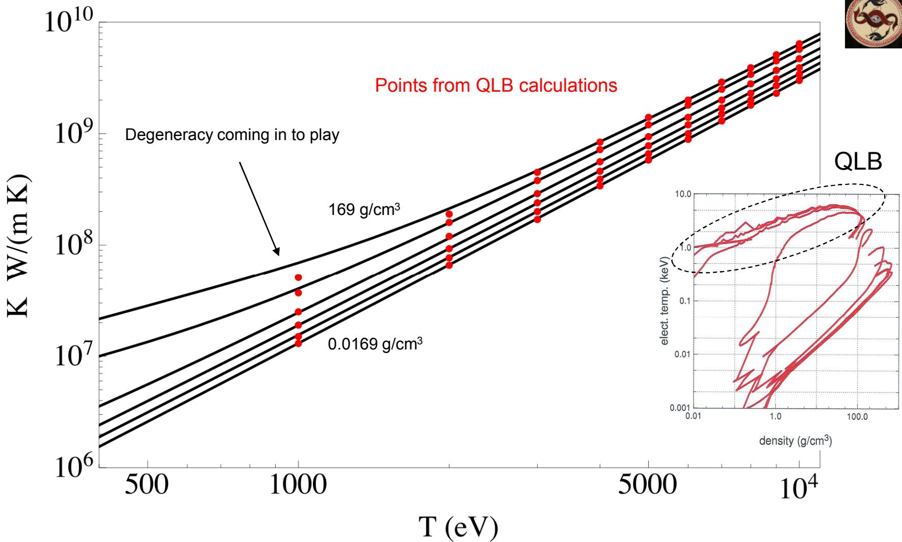
These QLB results are lower than the current LLNL thermal conductivity model by about 15%
