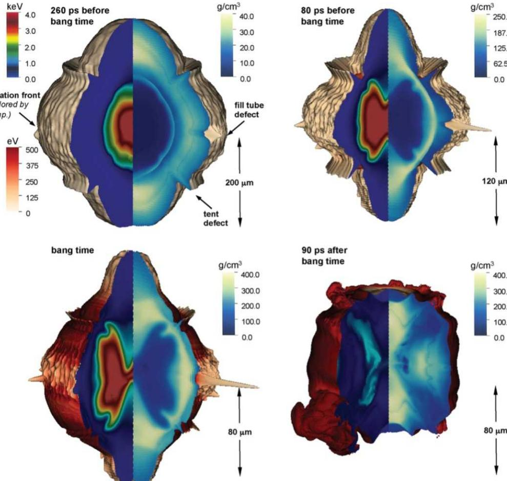
Simulations of NIF high-foot capsule implosions with lowered thermal conductivity are in better agreement with experiment
