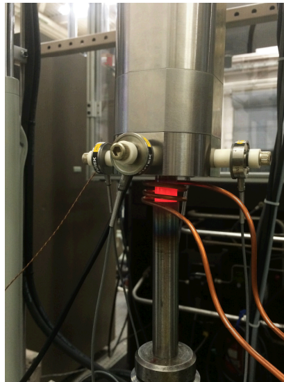
Fig. 8 Photograph showing induction heating of threaded rod and specimen.
