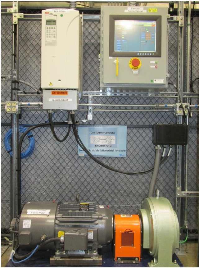
Figure 6: The mechanical source emulator is shown with ABB ACS800 drive, custom programmable feedback controller, Baldor 15 HP induction motor, and 10 kW SDW-PMSM installed with two 3-phase windings. The emulator is programmed to emulate the dynamics of a gas-turbine generator.
