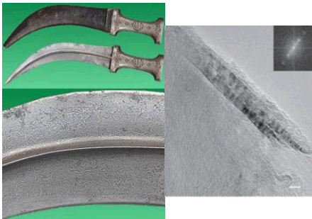
Carbon nanotubes in 17 th Century Damascus steel
