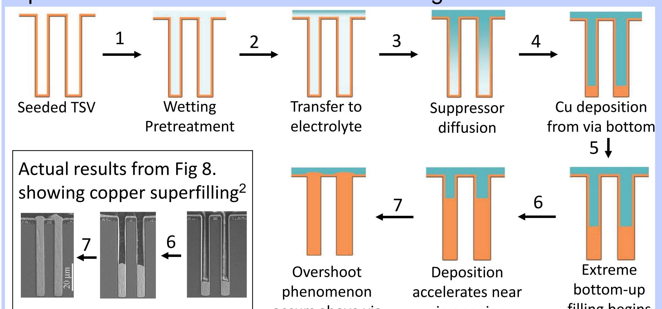
Electrolytes exhibiting S-NDR show hysteresis in cyclic voltammograms due to breakdown of adsorbed suppressor. Deposition at potentials in the hysteretic region produces 'Turing patterns' with active and passive regions:<sup>2</sup>
