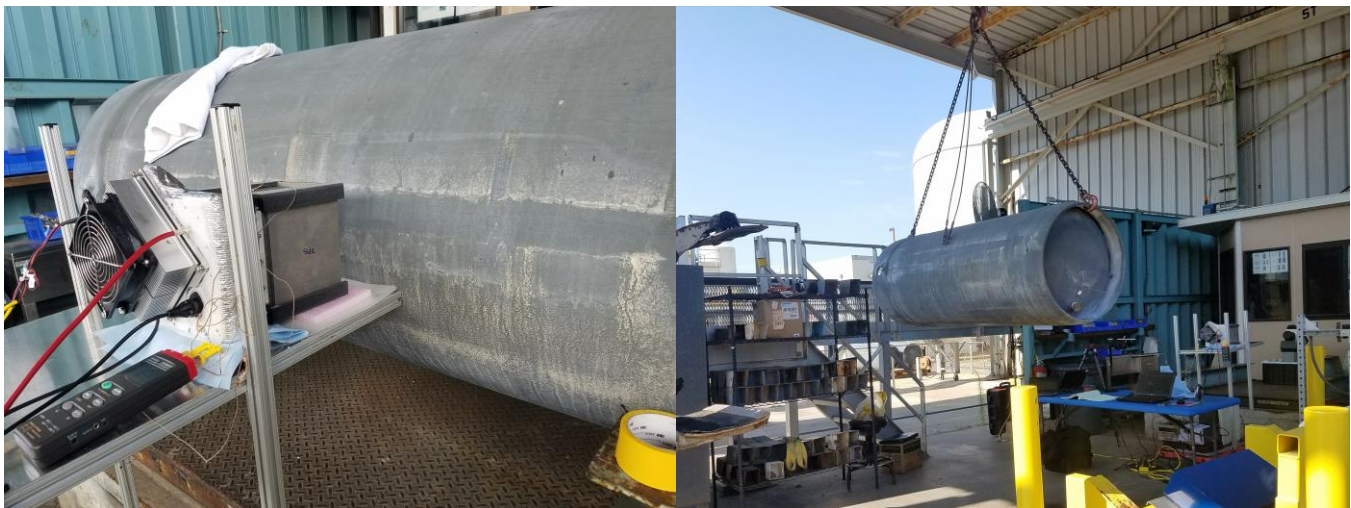
Figure 7. Placement and measuring point of UF 6 cask with the linear array detector. The rightmost image displays the changing of casks in between measurements.
