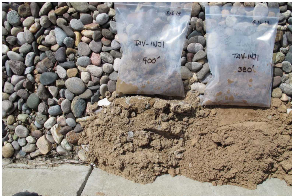
Figure B-6 Photograph of cuttings from injection well TAV-INJ1. From right to left 380 and 400 feet below ground surface.
