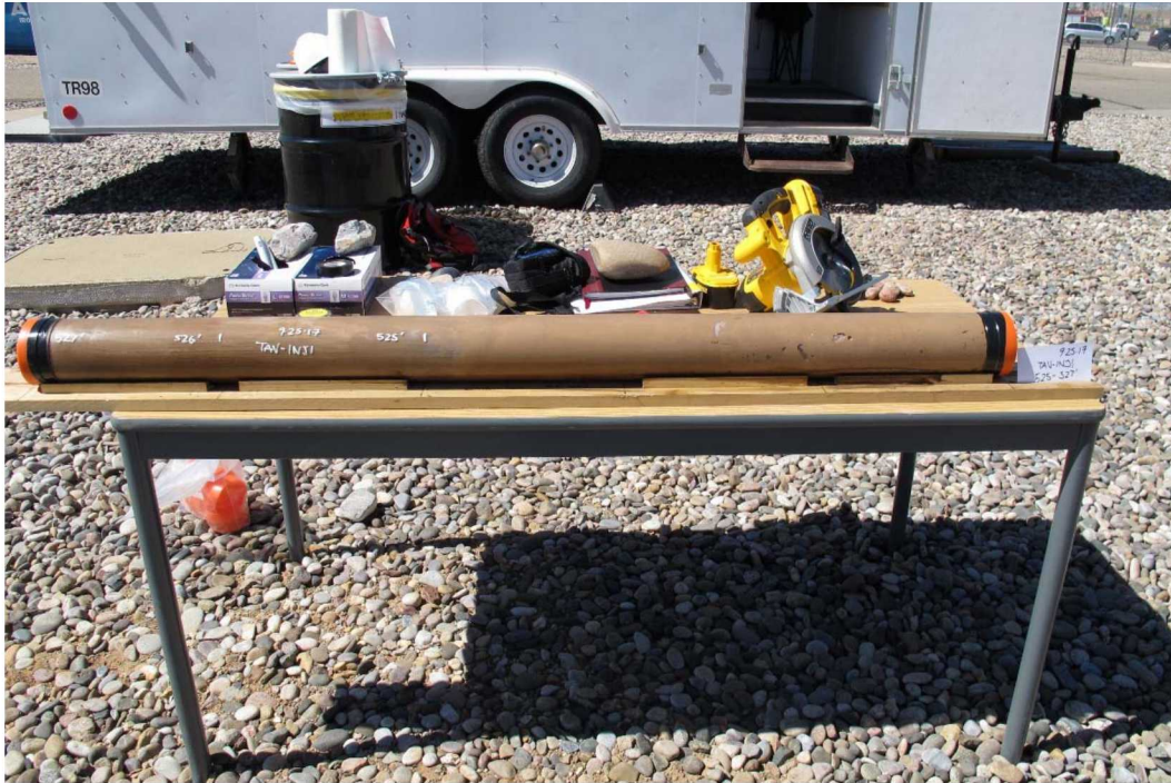
Figure C-7 Photograph of continuous core sample from monitoring well TAV-INJ1. From right to left the sample was from 525 to 527 feet below ground surface.
