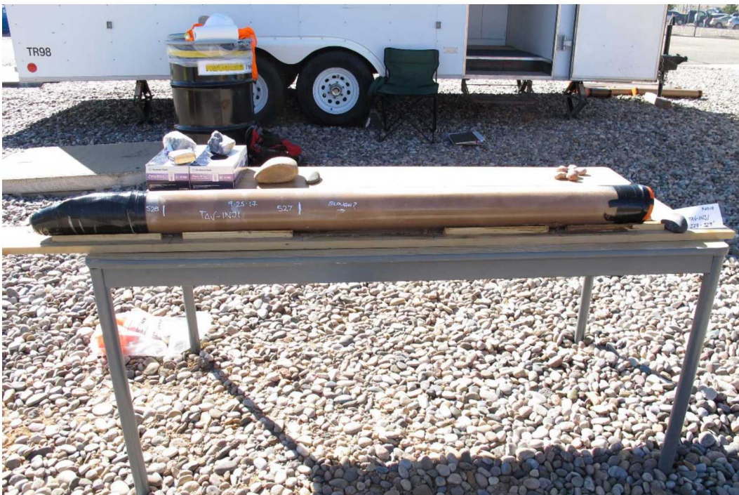
Figure C-8 Photograph of continuous core sample from monitoring well TAV-INJ1. From right to left the sample was from 527 to 529 feet below ground surface.
