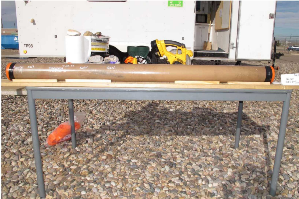
Figure C-4 Photograph of continuous core sample from monitoring well TAV-INJ1. From right to left the sample was from 508.5 to 510 feet below ground surface.
