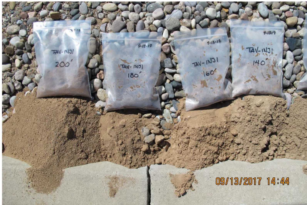
Figure B-3 Photograph of cuttings from injection well TAV-INJ1. From right to left 140, 160, 180, and 200 feet below ground surface.
