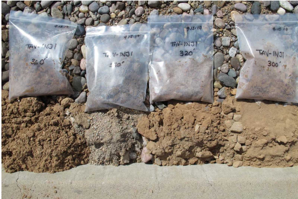
Figure B-5 Photograph of cuttings from injection well TAV-INJ1. From right to left 300, 320, 340, and 360 feet below ground surface.
