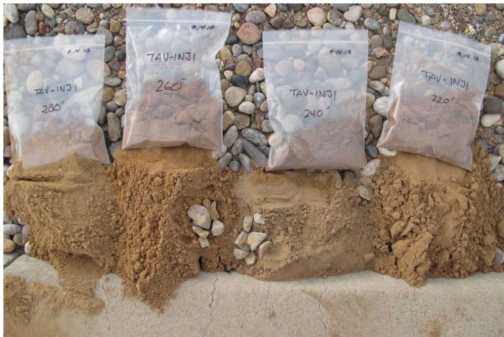
Figure B-4 Photograph of cuttings from injection well TAV-INJ1. From right to left 220, 240, 260, and 280 feet below ground surface.
