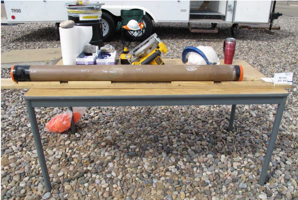
Figure C-3 Photograph of continuous core sample from monitoring well TAV-INJ1. From right to left the sample was from 505 to 508.5 feet below ground surface.
