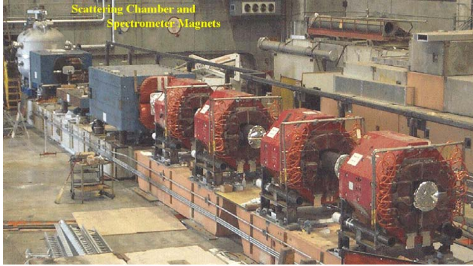
Figure 11: Scattering chamber for the \text{LH}_2 target and spectrometer magnets (2 of 3 dipoles for the chicane, and 4 quadrupoles) during beamline construction in End Station A.
