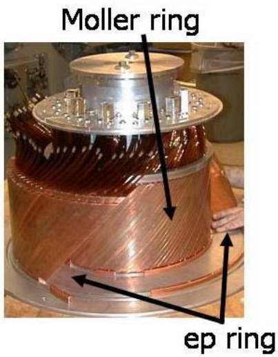
Figure 18: MOLLER-ep Detector during assembly.
