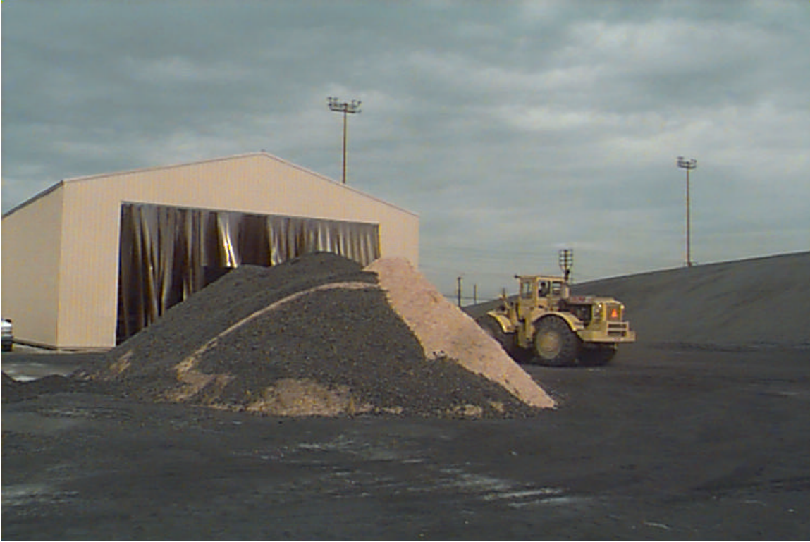
Figure 10. Blending Wood Waste and Coal for Cofiring at Bailly Generating Station
