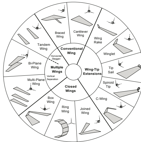
Figure 1: Different nonplanar wing designs. Box-wings are a member of the closed nonplanar wing family [3].
