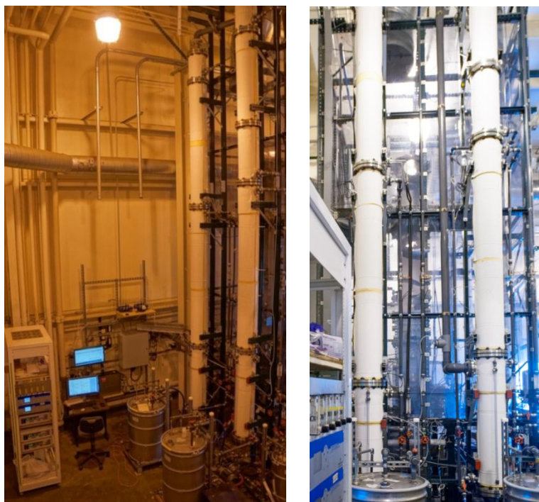
Figure 15. Photograph of the installed mixed salt absorber system ( left ) and close up of two absorber columns ( right ).
