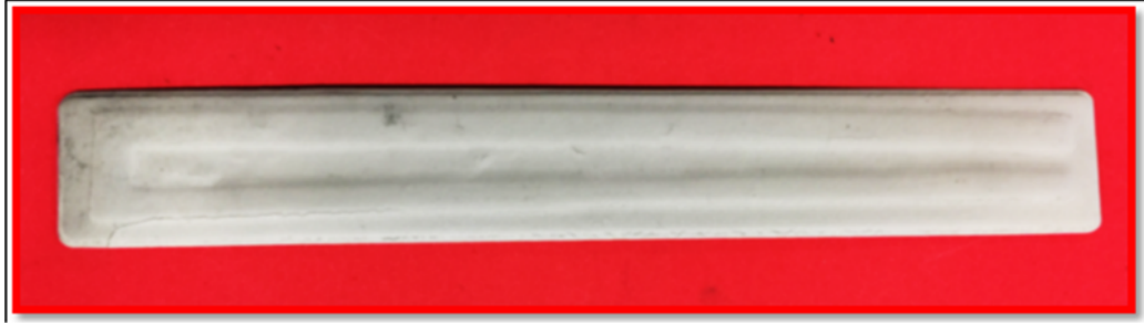
Figure 3.40. Photograph of [75-25] vol% \text{WSi}_2\text{-Al}_2\text{O}_3 thermistors embedded in fine alumina and sintered at 1600 °C for 5h in argon atmosphere.
