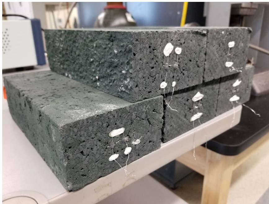
Figure 7.4. Full-size bricks with embedded LNO-1400 preforms and attached platinum wire leads.
