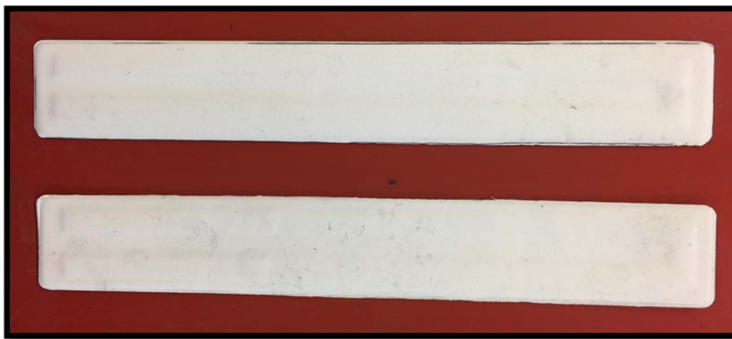
Figure 3.39. Photograph of [75-25] vol% WSi 2 -Al 2 O 3 thermistor green preforms embedded in fine alumina (SA: 8.6 m 2 /g) substrates (length 8 ¾” and thickness ~650 μm).
