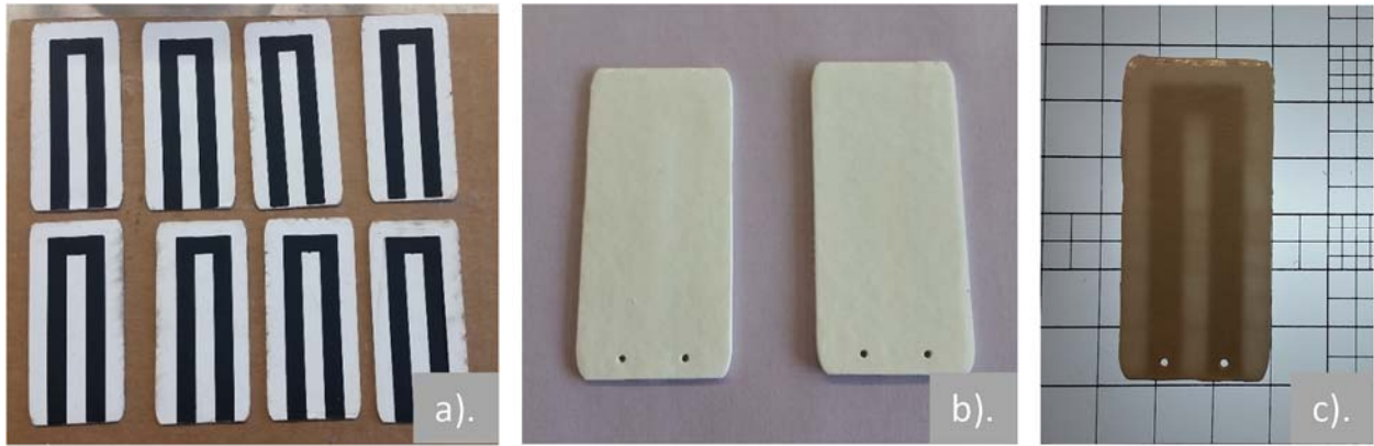
Figure 3.44 Images showing LNO thermistors: a) green, b) sintered, and c) sintered imaged on a light box to highlight embedded sensor material.
