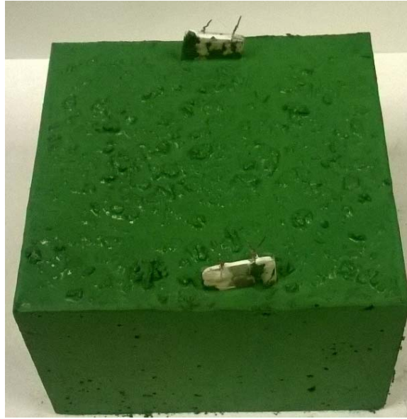
Figure 4.2. Chromia brick showing the embedded sensor.
