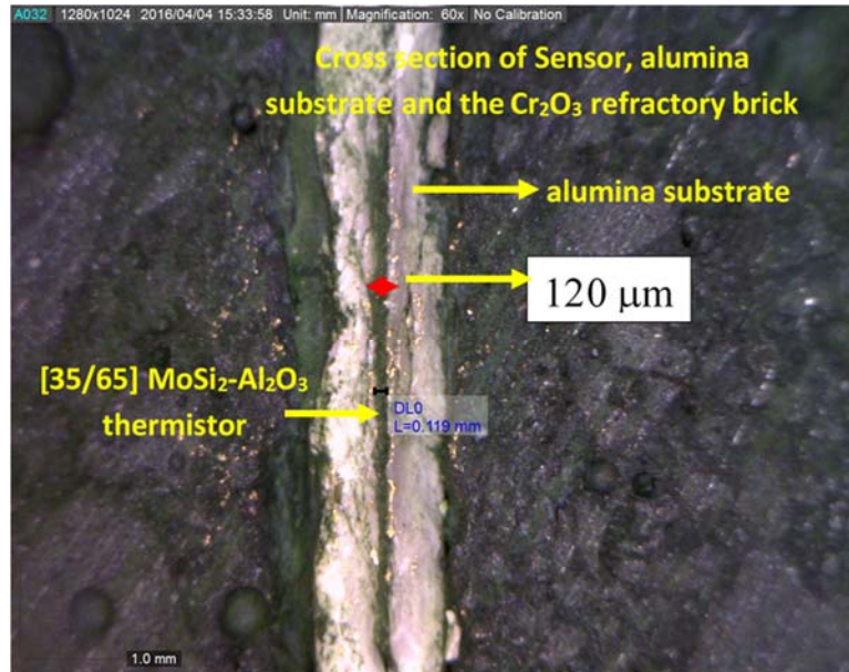
Figure 4.6. Optical micrograph of the cross sectional interface of the smart brick embedded with [35-65] vol. % \text{MoSi}_2\text{-Al}_2\text{O}_3 long thermistor.
