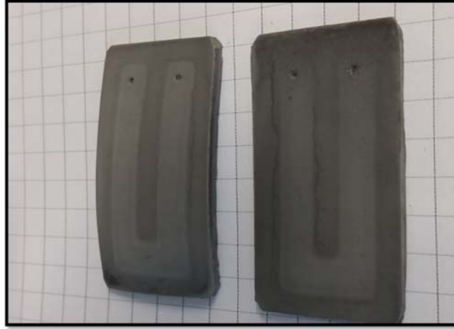
Figure 3.5. Photograph of [30-70] \text{MoSi}_2\text{-Al}_2\text{O}_3 thermistor (with material) embedded in fine alumina substrates and sintered at 1600^\circ\text{C} for 2h in argon atmosphere.
