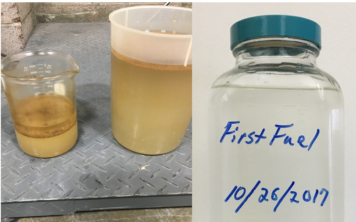
Figure 10. FT first oil and produced water at Ceramatec, October 26, 2017.
