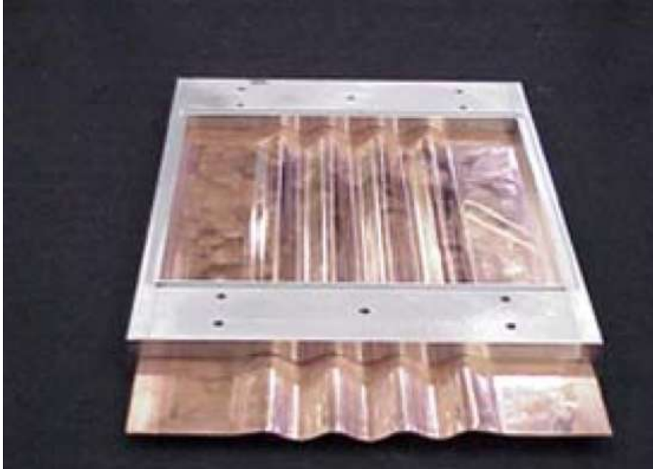
Fig. 2.6 Sinusoidally shaped copper plate and support frame (from Fig. 1 of Puranik et al., 2004, with permission from Shock Waves ).
