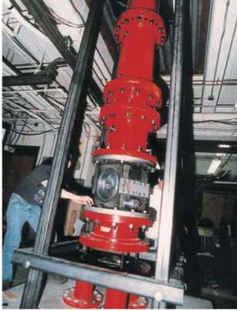
Fig. 7.3 (Anderson et al., 2000, Shock Waves , with permission). The Wisconsin vertical shock tube.
