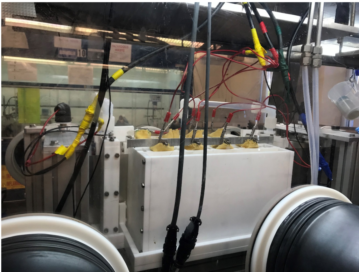
Figure 16. Reel to reel plating system installed in the glovebox environment.
