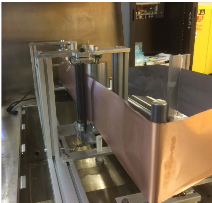
Figure 13. Continuous thickening station for reel to reel plating on nano-Al.
