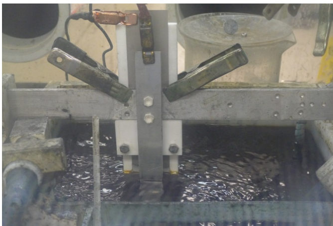
Figure 6. 20 liter plating reactor for nano-Al used to produce 2x2 inch sheet samples as part of the scale-up effort.
