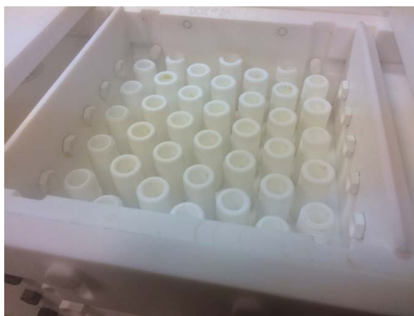
Figure 10. 6x6 inch flow cell showing the adjustable nozzle configuration.
