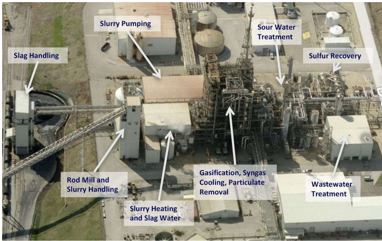
Figure 3. Aerial view of the QSG facility with various components of the syngas to ammonia process. The Acid Gas Recovery system is associated with the Sulfur Recovery location.
