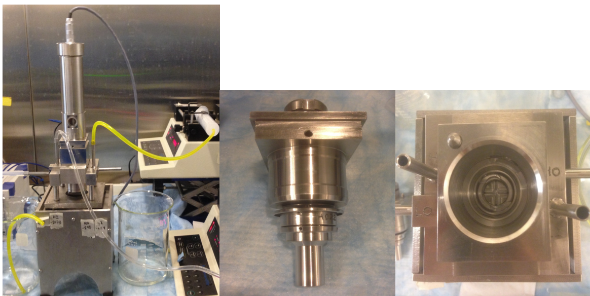
Figure 20. Left, Robatel BXP012 contactor with syringe pump. Middle, rotor. Right, Stationary housing.
