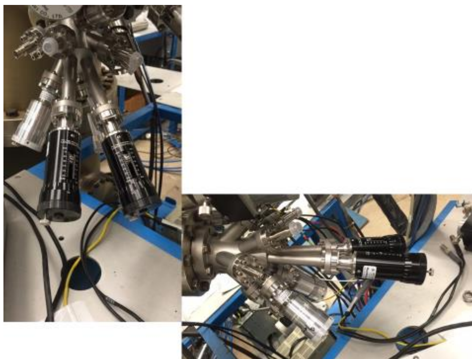
Fig. 15. The e-beam evaporation cell installed on the MBE system.
