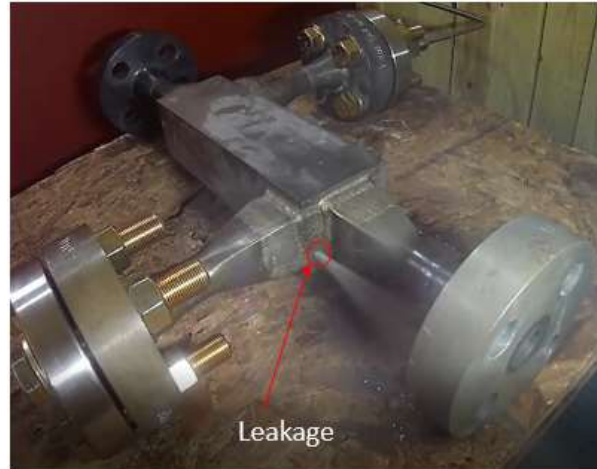
Figure 193. The leakage of the PCHE during the second test
