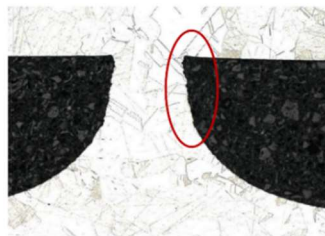
Figure 104 A micro-scale image of zigzag channels with smooth roundness at the bottom and adjacent rougher area (Southall et al. 2009)
