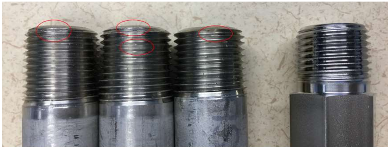
Figure 150. Defective threads on pipe nipples (left) and high-quality threads on the pipe nipple from Hy-lok (right)
