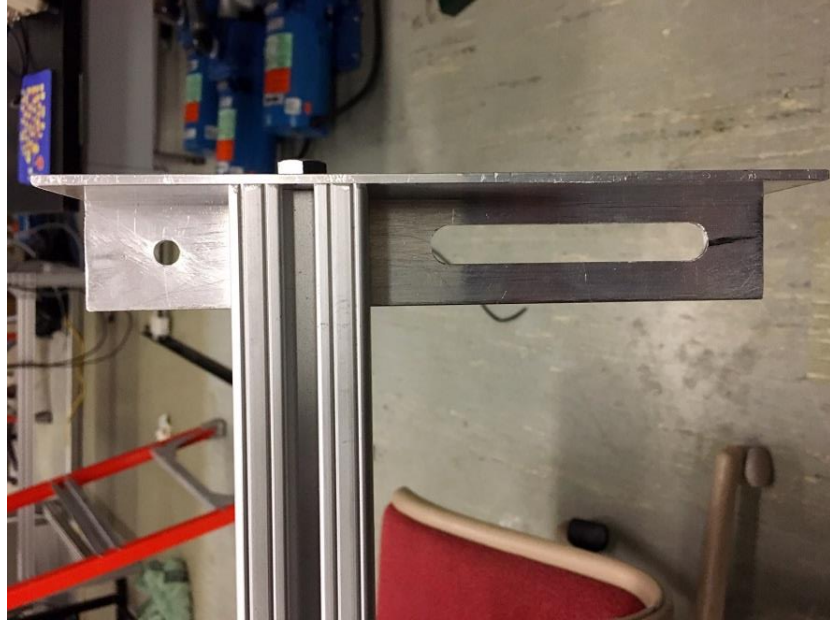
Figure 17. Slots on the shoulders of the target holder.
