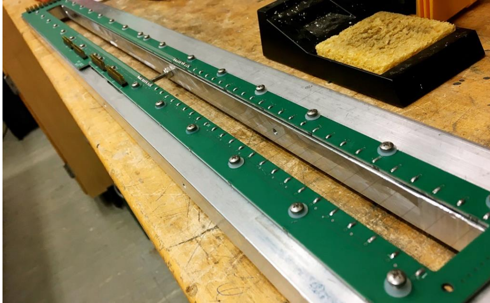
Figure 22. Wire-mesh sensor mounted on the frame in ECMFL.
