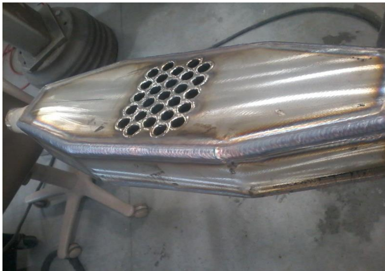
Figure 2.26 Facility with tube bank welded
