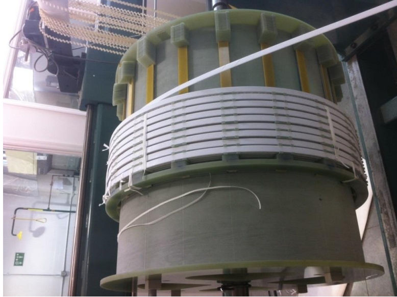
Figure 2.3.1.5.1 Winding of HV module with insulated clad HTS superconductor.
