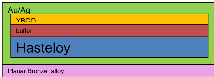
Figure 2.3.2.2.5 – Composite conductor configuration with planar sputtered bronze alloy
