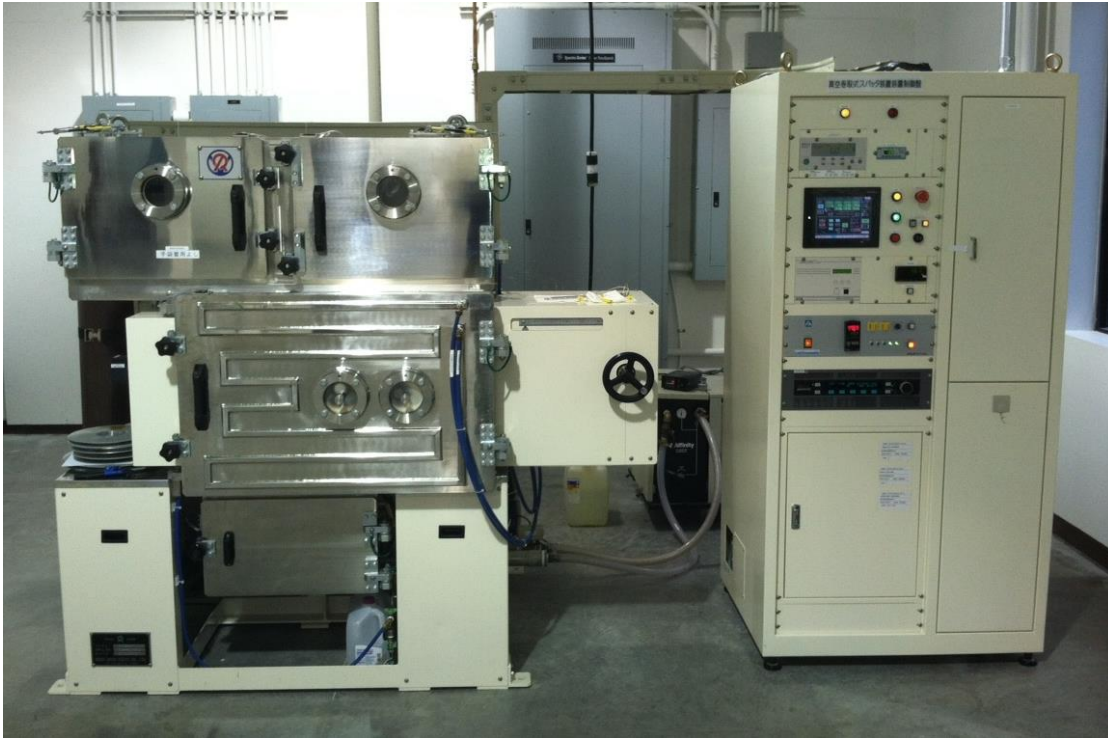
Figure 2.3.2.3.2 – Planar sputtering equipment used to deposit ~1.5 micron thick CuNi bonding layer on the Hastelloy side of the HTS tape.
