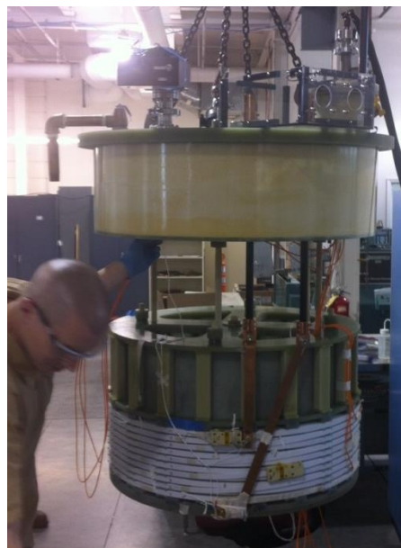
Figure 2.3.2.1.5 - Top plate of dewar with transformer HV scaled coil module in place for ac loss testing
