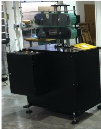
Figure 2.3.2.3.8 – Tractor drive used to provide tension in the line.
