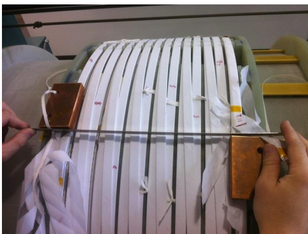
Figure 2.3.2.3.21 – a) Prototype termination, b) examples of terminations incorporated on test winding.
