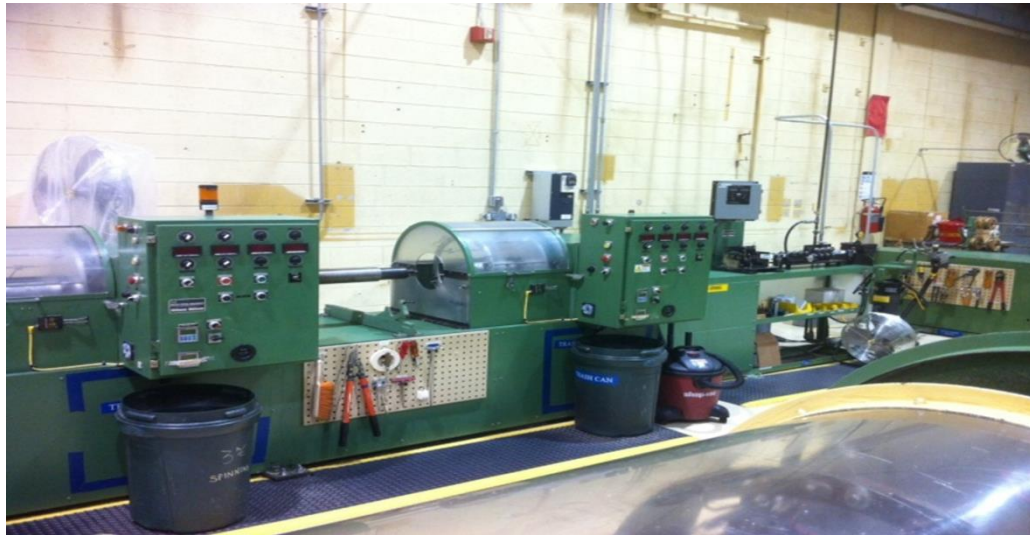
Figure 2.3.2.3.17 – Photo of reel-to-reel insulation system used to insulate thick clad product.
