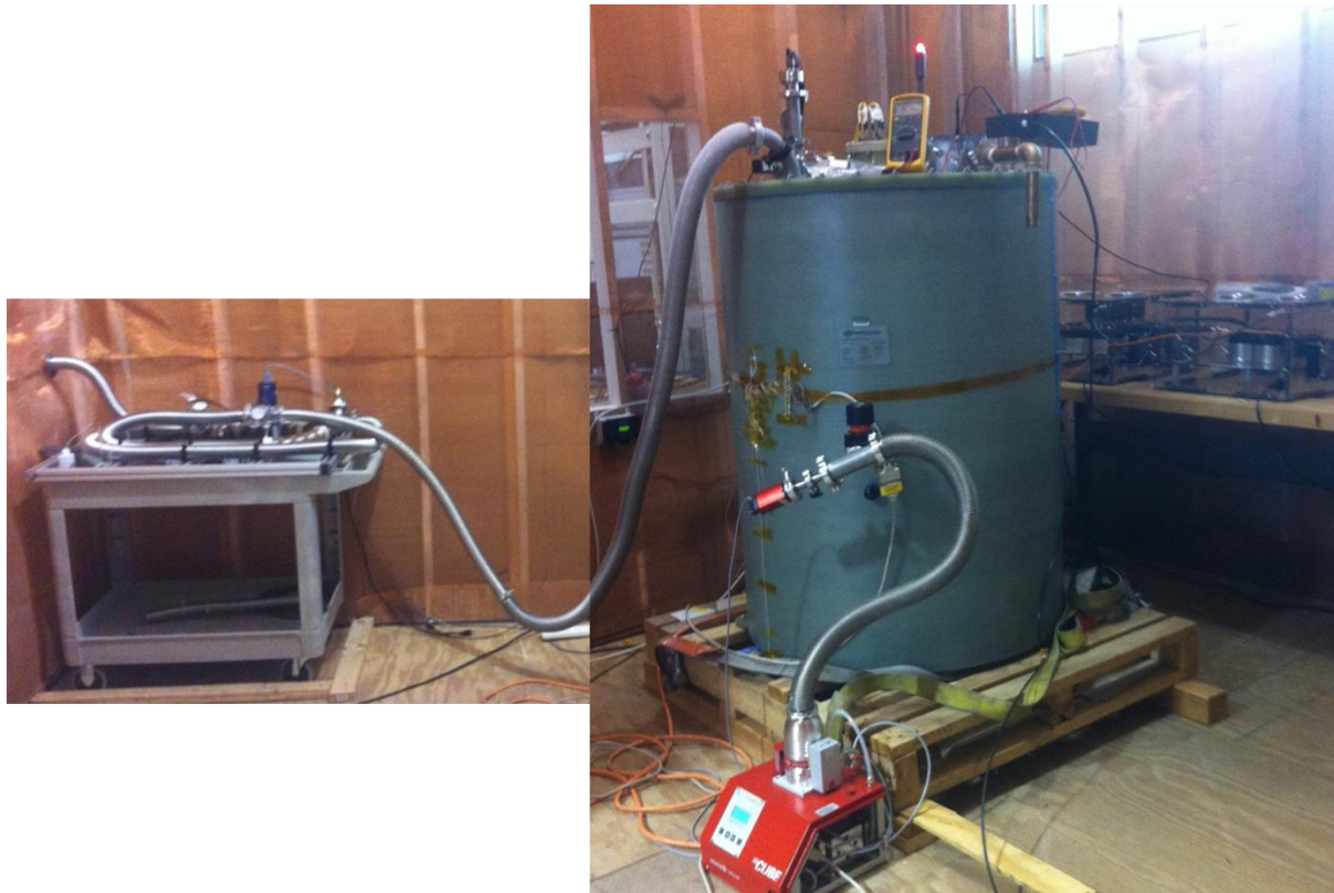
Figure 2.3.2.1.4 – Calorimetric ac loss test system for coils consisting of a double wall non-metallic vacuum insulated dewar (right) and a gas warming / mass flow meter system (left).
