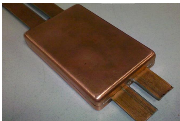
Figure 2.3.2.3.21 – a) Prototype termination, b) examples of terminations incorporated on test winding.
