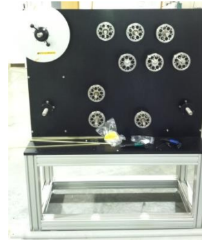
Figure 2.3.2.3.5 – Pay-off equipment for laminate (left) and HTS conductors (right).
