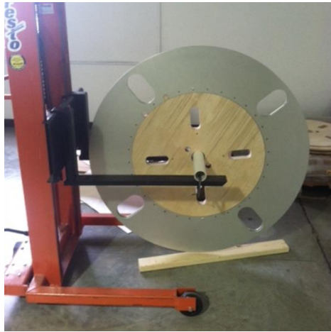
Figure 2.3.2.3.19 – Photo of handling equipment developed for the large spools carrying final insulated, clad product. \
