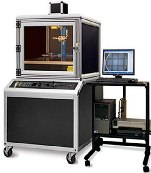
Figure 2.3.2.3.13 – X-ray system incorporated into the bonding line to evaluate solder voids in bonded product.
