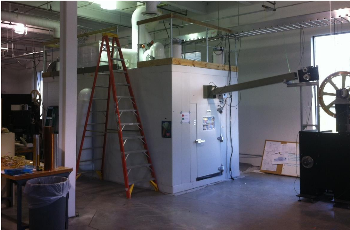
Figure 2.3.2.3.16 – Photo of reel-to-reel Ic test system for thick clad product.
