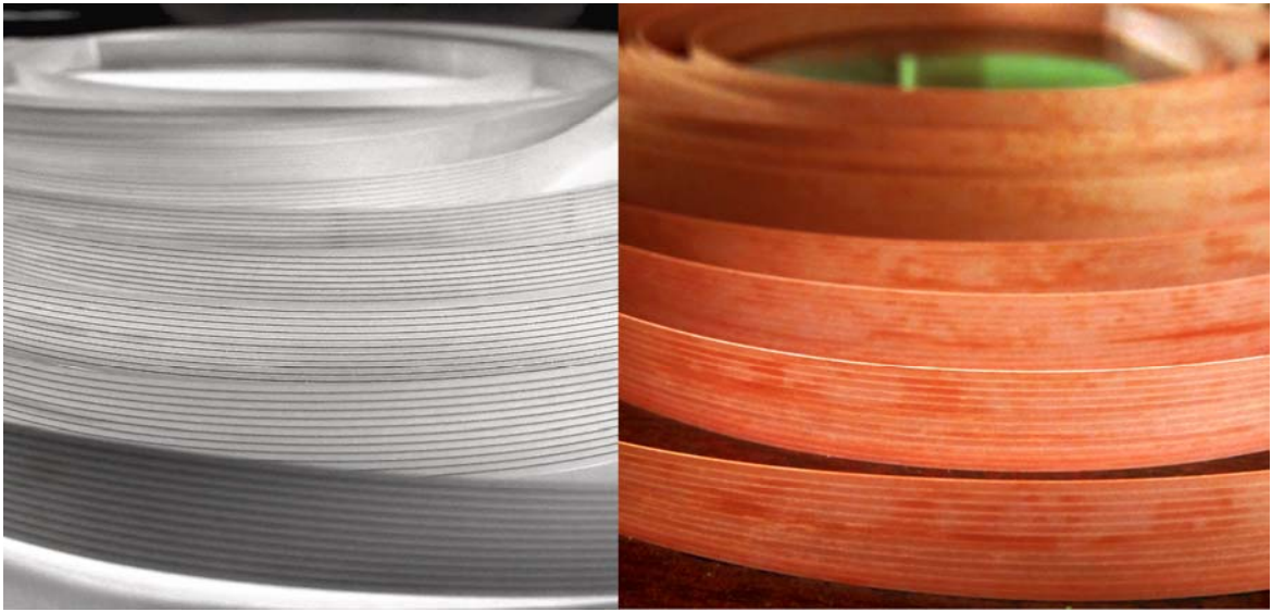
Figure 5: Reel to reel striated 10 m tape before copper electroplating (left) and after copper electroplating (right).
