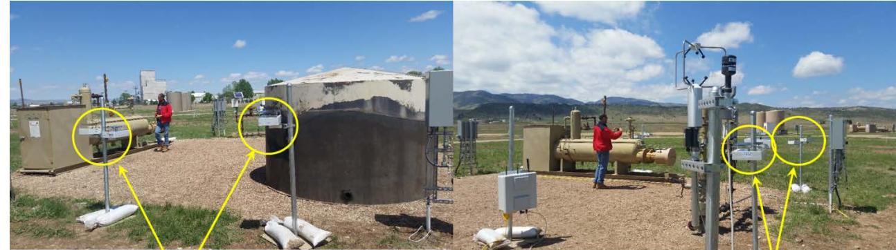
base station wind sensors methane sensors
