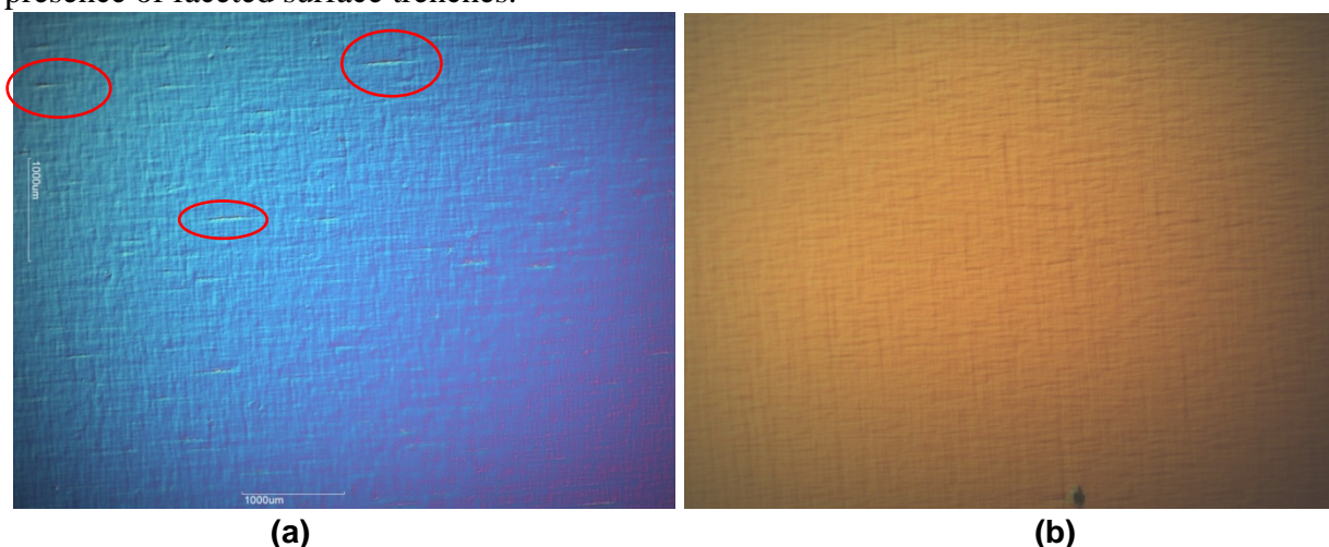
Figure 6: Nomarski optical microscope images of tensile \text{GaAs}_{0.9}\text{P}_{0.1} step graded buffers grown on Si with varying temperature profiles. (a) Constant temperature of 725°C and (b) 2-step temperature profile 725°C/650°C with lower temperature after \text{GaAs}_{0.5}\text{P}_{0.5} .
